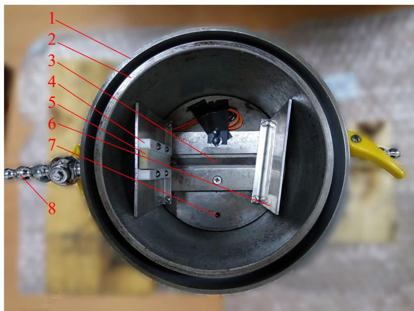
**Figure 2.** Inside view of AO cell: 1—external wall; 2—internal wall; 3—optical window; 4—sound transducer holder; 5—sound transducer; 6—sound reflector; 7— $\text{SF}_6$  gas inlet/outlet; 8—cooling water inlet/outlet.
