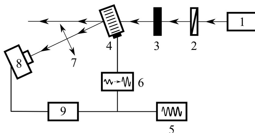
**Figure 1.** Schematic diagram of experimental setup: 1—FEL; 2—wire-grid polarizer; 3—set of calibrated radiation attenuators; 4—AO cell; 5—signal generator; 6—electrical amplifier; 7—lens; 8—Golay cell; 9—lock-in amplifier.
