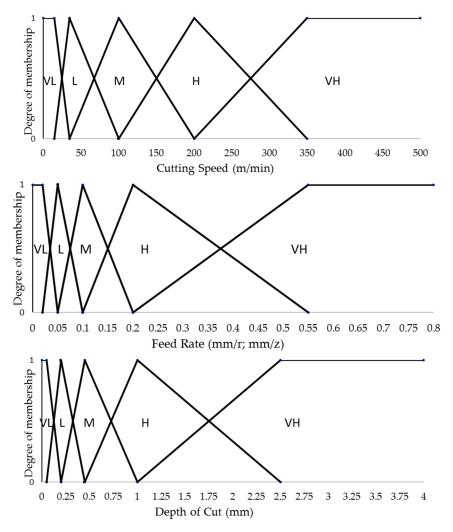
Figure 2. Fuzzy sets for the numeric control parameters of machining.
