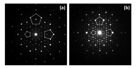
**Figure 5.** Comparison of electron diffraction patterns in [010] zone axis: decagonal quasicrystal in Al–Co-Cu system (**a**),  $\varepsilon_{16}$  decagonal quasicrystalline approximant in Al–Pd–Co system (**b**).
