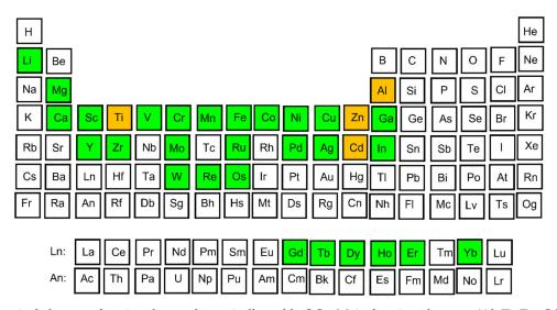
**Figure 1.** Chemical elements forming thermodynamically stable QCs. Main forming elements (Al, Ti, Zn, Cd) are marked by orange color, alloying elements are denoted by green.
