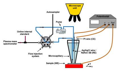
Figure 13. Schematic of the microcapillary flow ICP MS setup, re-drawn from reference [91].
