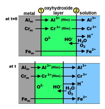
**Figure 14.** Schematic of the passive film evolution on  $\gamma$ -phase Al<sub>64.2</sub>Cr<sub>27.2</sub>Fe<sub>8.1</sub> alloy, re-drawn from reference [91].
