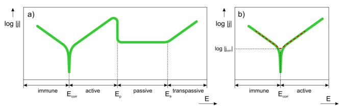
Figure 8. Schematic polarization curve of a passivating metal: (a) full curve, (b) Tafel extrapolation of cathodic and anodic regions.
