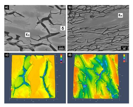
**Figure 18.** Microstructure of as-corroded Al–Pd–Co alloys: backscatter scanning electron microscopy images of  $Al_{70}Pd_{25}Co_5$  (**a**) and  $Al_{74}Pd_{12}Co_{14}$  (**b**) and confocal laser scanning images of  $Al_{70}Pd_{25}Co_5$  (**c**) and  $Al_{74}Pd_{12}Co_{14}$  (**d**). Reproduced from reference [107].
