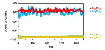
**Figure 17.** Open circuit potentials of Al–Pd alloys in aqueous NaCl, re-plotted from data in reference [105].
