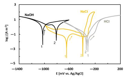
**Figure 12.** Potentiodynamic cyclic polarization curves of near-equilibrium Al<sub>74</sub>Co<sub>26</sub> alloy in different electrolytes, re-plotted from reference [86].
