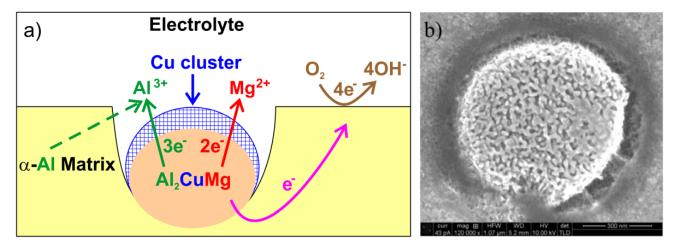
**Figure 10.** Schematic of trenching of  $Al_7Cu_2Fe$  intermetallic in AA2024-T3 aluminum alloy (**a**); microstructure image of corroded alloy surface after 1-h exposure in aerated  $H_2O$  at 30 °C, redrawn (**a**) and reproduced (**b**) from ref. [76].
