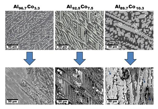
**Figure 11.** Microstructure of the rapidly solidified Al–Co alloys before and after corrosion in aqueous NaCl, adapted from reference [81].
