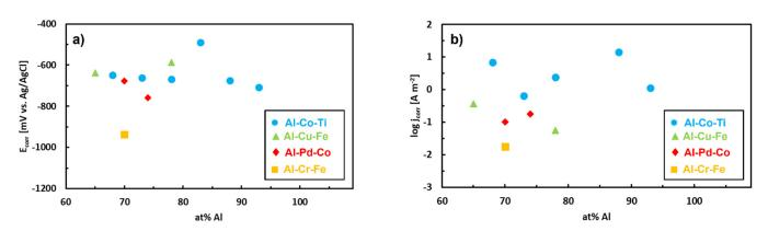
**Figure 20.** Corrosion parameters of ternary Al–TM alloys in aqueous NaCl ( $0.6 \text{ mol L}^{-1}$ ). Data is compiled from references [90,107,109,110].
