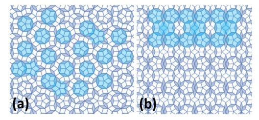
**Figure 4.** Schematic structure of quasicrystal (a) and quasicrystalline approximant (b) with denoted star-shape corresponding to clusters in real structure. Quasicrystalline arrangement is represented by Penrose tiling.
