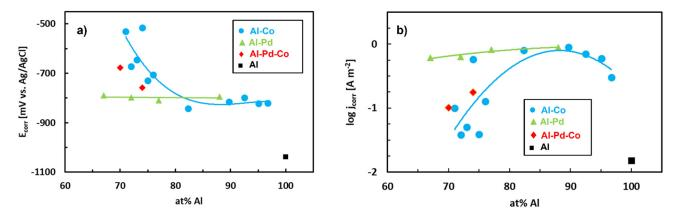
**Figure 19.** Corrosion parameters of Al–Pd, Al–Co and Al–Pd–Co alloys in aqueous NaCl ( $0.6 \text{ mol L}^{-1}$ ). Data is compiled from references [81,82,84,105,107].
