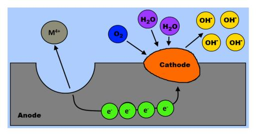
Figure 6. An elementary electrochemical corrosion cell on metal surface.
