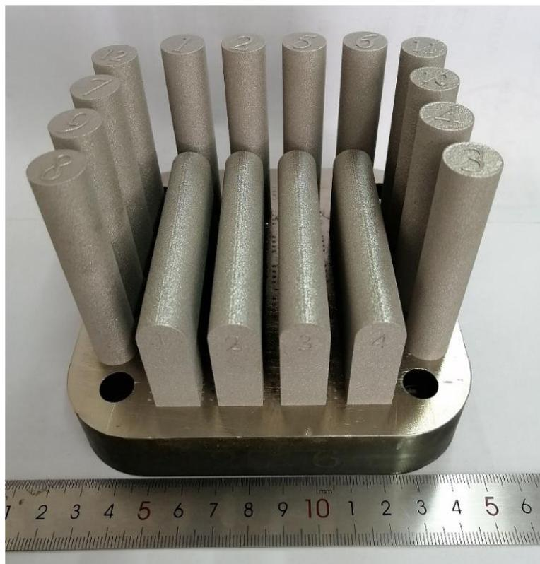
**Figure 2.** The size and distribution of the SLM processed samples.
