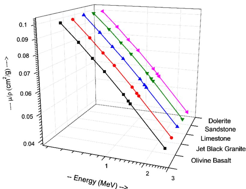
Figure 2. Mass attenuation coefficient ( $\mu/\rho$ ) obtained by EPICS2017 of the natural rocks at the 0.37–2.51 MeV region.
