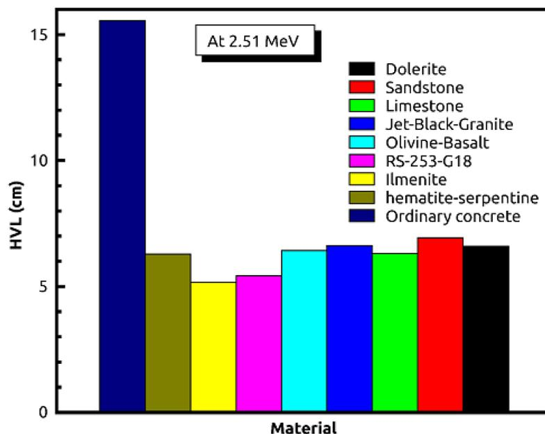
**Figure 6.** Comparison of the natural rocks with common shielding materials in terms of HVL at 2.51 MeV.
