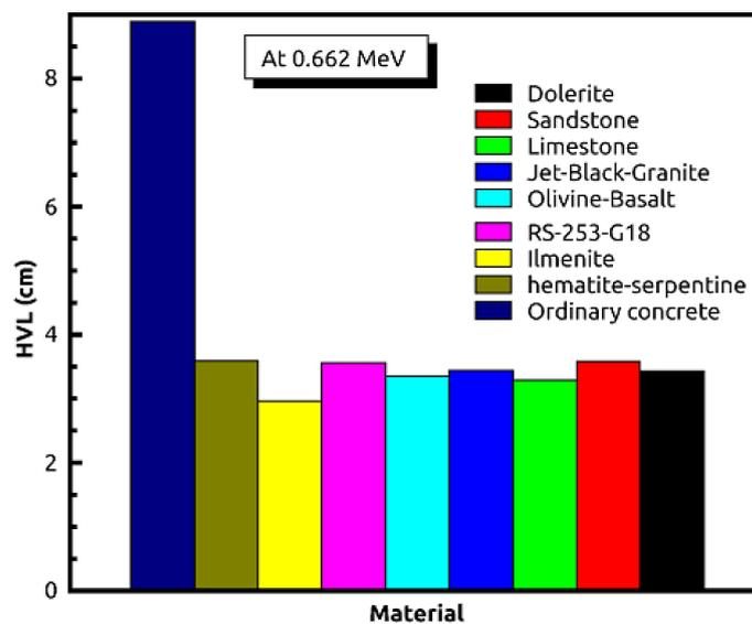
Figure 5. Comparison of the natural rocks with common shielding materials in terms of HVL at 0.662 MeV.
