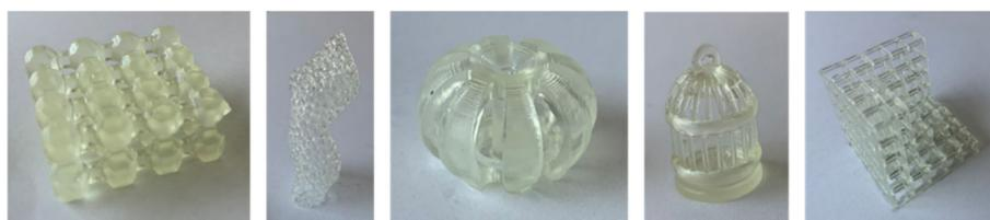
**Figure 10.** Complex-shaped objects printed from E40DGMA60. No thermal treatment is applied. From left to right: zeolite structure, fish-net woman, fountain light, bird cage, perforated cube (staggered).
