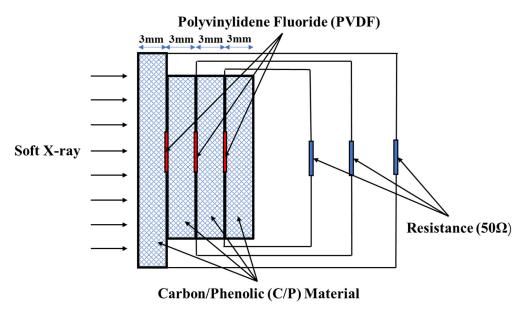
Figure 2. A schematic diagram of PVDF thermal shock wave stress measurement.
