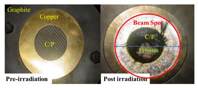
Figure 3. Experimental photos before and after X-ray irradiation.
