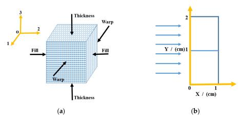
**Figure 6.** Schematic diagrams of the C/P material model: (a) principal directions and lamina of the composite and (b) a simplified model for the numerical simulation.
