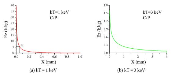
**Figure 7.** The deposited energy distribution along the symmetry axis under irradiation of X-ray with different blackbody spectra. (a) kT = 1 keV; (b) kT = 3 keV.
