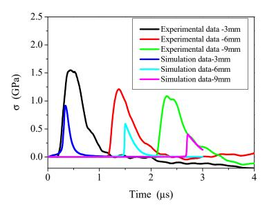
**Figure 5.** A comparison of C/P material experiment and calculation data.
