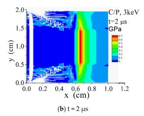
Figure 10.  $\sigma xx$  (GPa) contours of C/P under radiation of X-ray with 3 keV blackbody spectrum. (a) t = 1 us; (b) t = 2 us.
