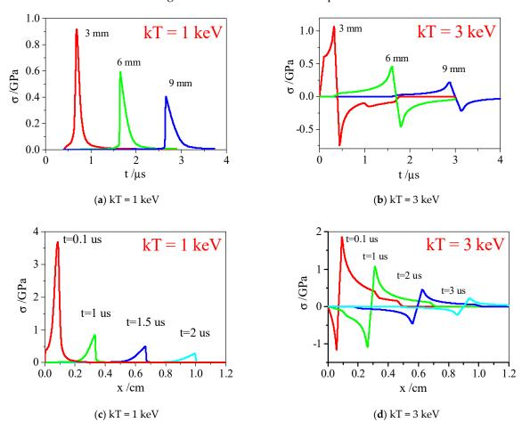
**Figure 8.** The stress wave along symmetry axis of C/P under radiation of X-ray with different blackbody spectra. (a) time distribution, kT = 1 keV; (b) time distribution, kT = 3 keV; (c) space distribution, kT = 1 keV; (d) space distribution, kT = 3 keV.
