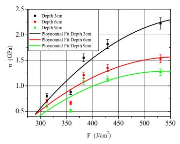
Figure 4. The measured peak stress of thermal shock wave and fitted peak attenuation curve.
