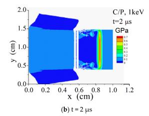
**Figure 9.**  $\sigma xx$  (GPa) contours of C/P under radiation of X-ray with 1 keV blackbody spectrum. (a) t = 1 us; (b) t = 2 us.
