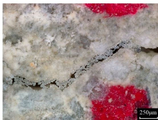
Figure 1. Irregular healing products on the crack surface.
