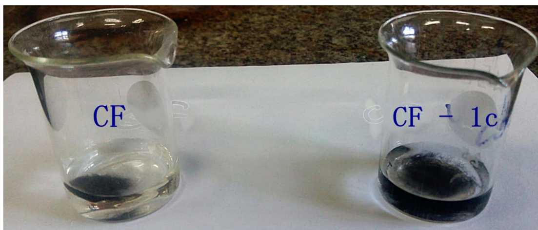
Figure S3. Photos showing the behavior of CF nonwoven and CF-1c nonwoven after incorporation of the rest of benzoic acid in water. Wettability test.
