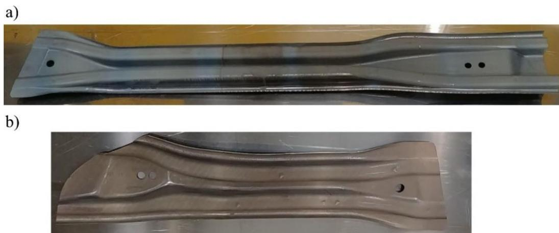
**Figure 20.** Drawpieces for door beams (a) long, (b) short.
