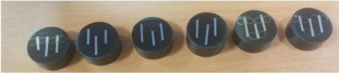
Figure 22. Ready-made samples prepared for testing, embedded in phenolic resin.
