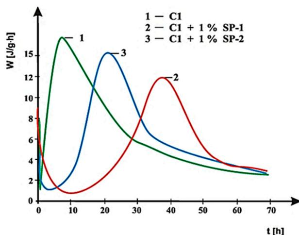
**Figure 21.** Hydration heat evolution rate curves for C1 cement without and with 1% by mass of SP-1 and SP-2 superplasticizers.
