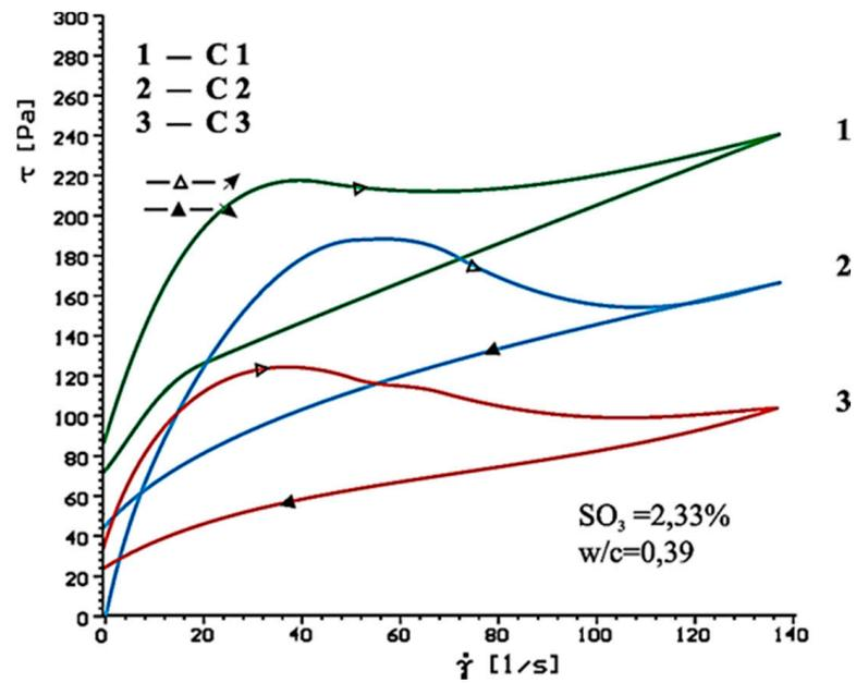
Figure 7. Flow curves of cement pastes with addition of  $\text{CaSO}_4 \cdot 0.5\text{H}_2\text{O}$ ,  $\text{CaSO}_4$ ,  $\text{CaSO}_4 \cdot 2\text{H}_2\text{O}$ , after 60 min.
