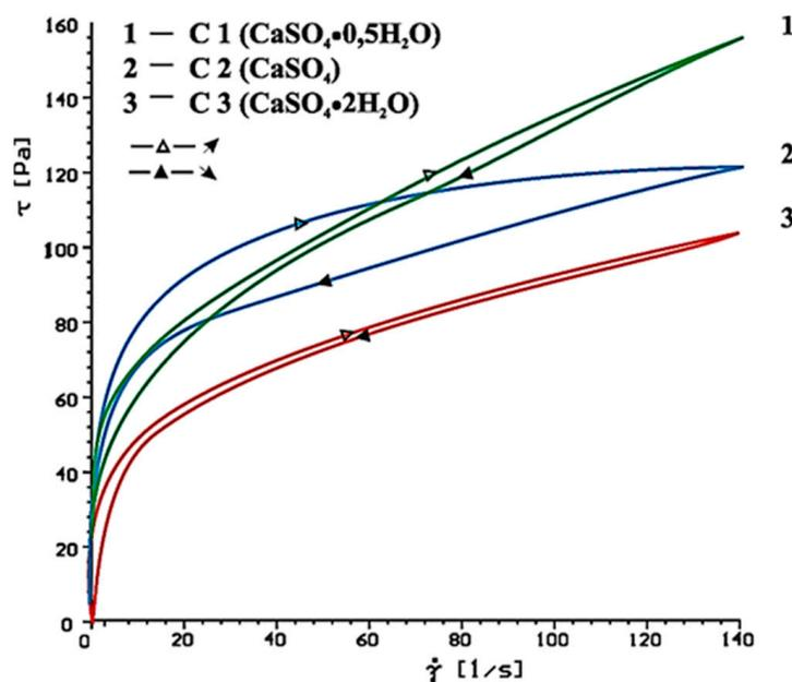
**Figure 6.** Flow curves of cement pastes with addition of  $CaSO_4 \cdot 0.5H_2O$ ,  $CaSO_4$ ,  $CaSO_4 \cdot 2H_2O$ , after 10 min.
