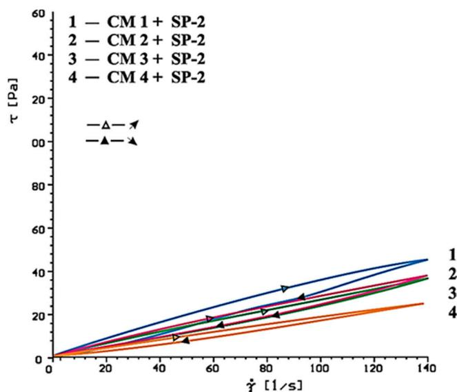
Figure 18. Flow curves of cementitious pastes containing 5% by mass of  $\text{CaSO}_4 \cdot 0.5\text{H}_2\text{O}$  and  $\text{CaSO}_4$  in quantity from 20 to 80% by mass in presence of SP-2 type superplasticizer, 1% by mass, after 10 min.
