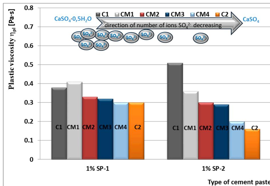
**Figure 20.** Plastic viscosity  $\eta_{pl}$  of pastes from cements C1, CM1, CM2, CM3 and C2 containing calcium sulphate anhydrite without and with 1% by mass of SP-1 and SP-2 superplasticizer, determined after 10 min.
