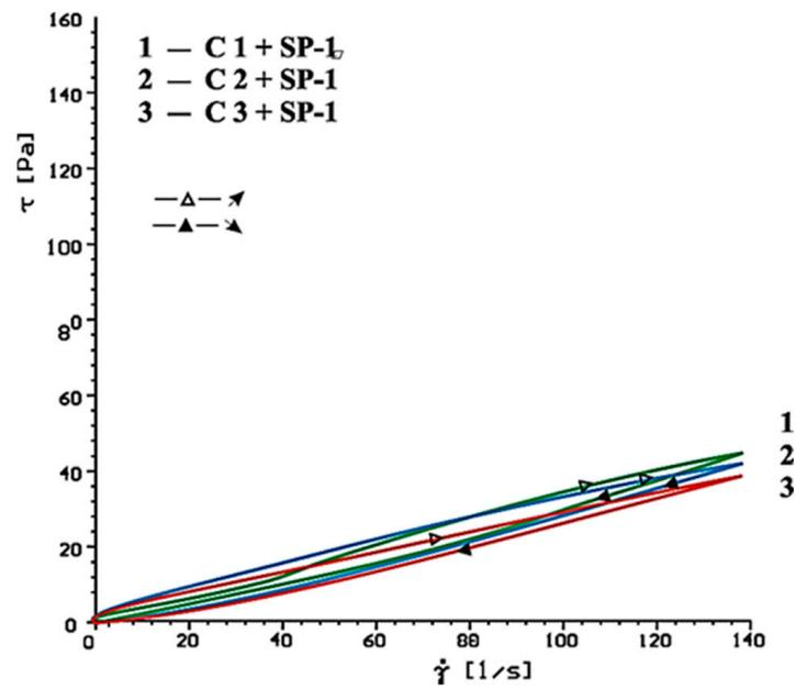
Figure 8. Flow curves of cement pastes with addition of  $\text{CaSO}_4 \cdot 0.5\text{H}_2\text{O}$ ,  $\text{CaSO}_4$ ,  $\text{CaSO}_4 \cdot 2\text{H}_2\text{O}$  in presence of SP-1 superplasticizer, after 10 min.
