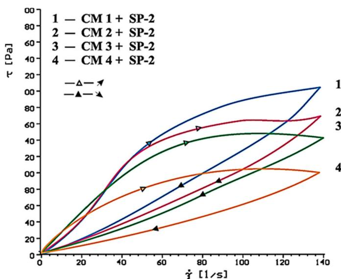
Figure 19. Flow curves of cement pastes containing 5% by mass of  $\text{CaSO}_4 \cdot 0.5\text{H}_2\text{O}$  and  $\text{CaSO}_4$  in quantity from 20 to 80% by mass in presence of SP-2 type superplasticizer, 1% by mass, after 60 min.
