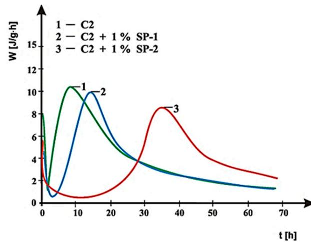
Figure 22. Hydration heat evolution rate curves for C2 cement without and with 1% by mass of SP-1 and SP-2 superplasticizers.
