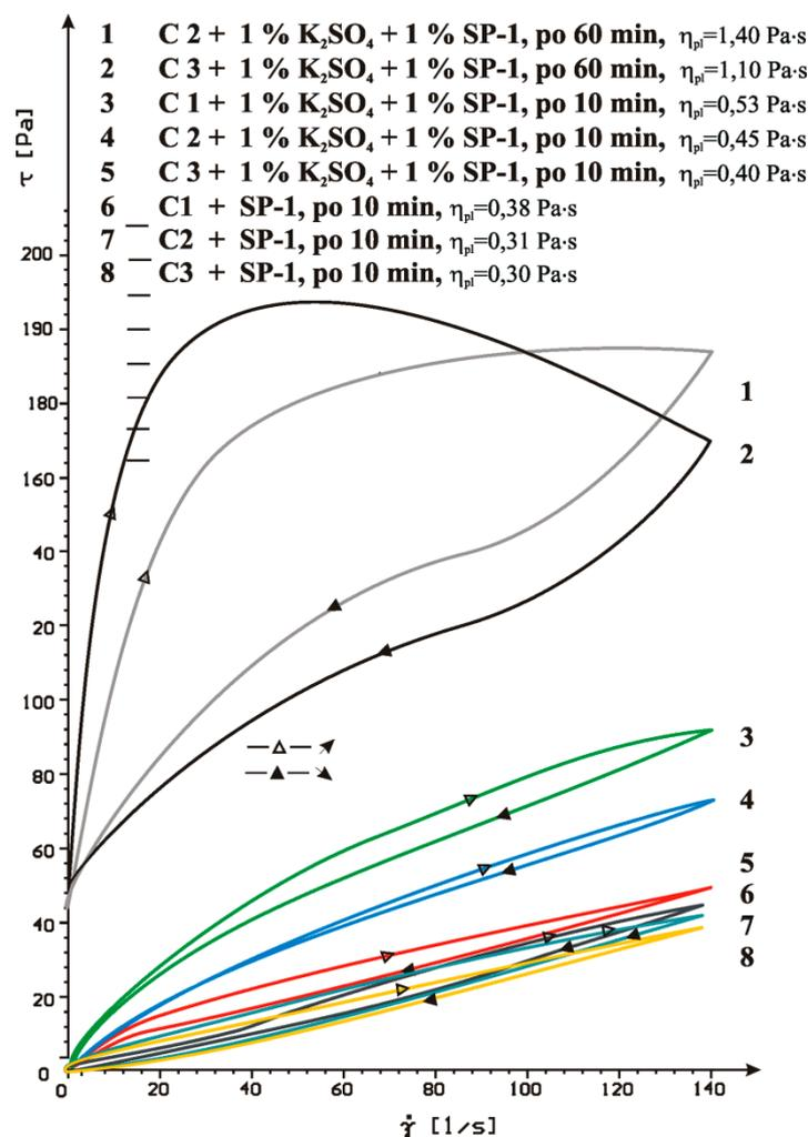
**Figure 12.** Flow curves of pastes of C1, C2 and C3 cements containing  $\text{K}_2\text{SO}_4$  in presence of SP-1 in 1% by mass, after 10 and 60 min.
