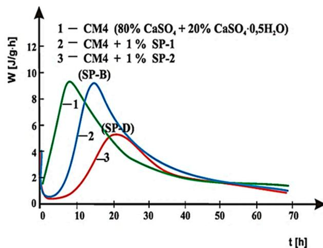
Figure 26. Hydration heat evolution rate curves for CM4 cement without and with SP-1 and SP-2 superplasticizers.
