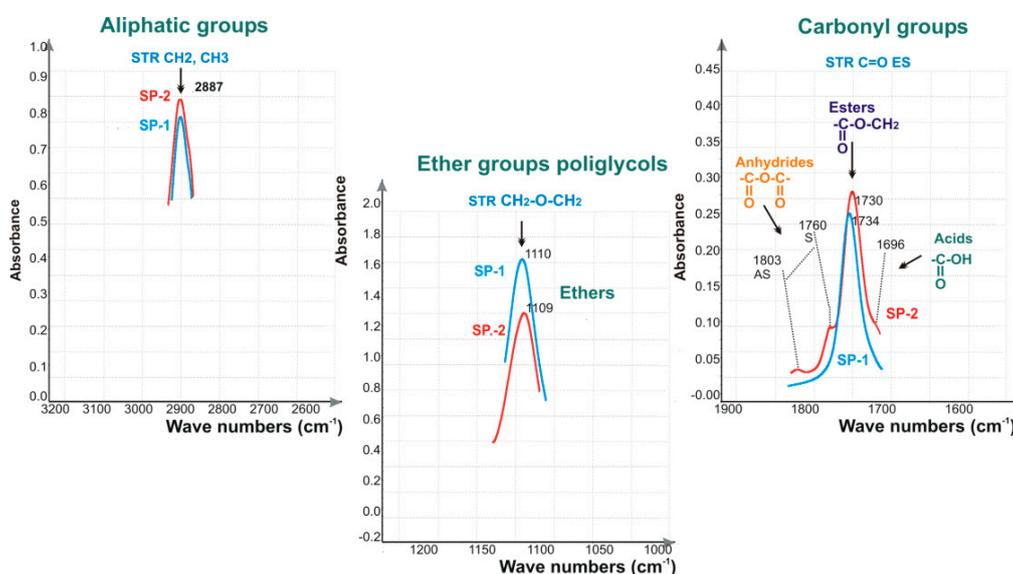
**Figure 3.** Selected function groups: Aliphatic, ether and carbonyl groups identified by means of IR testing), (based on results published in [41]).
