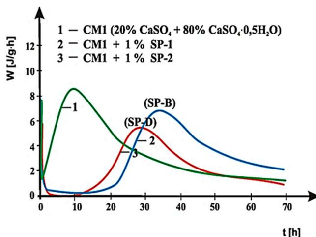
Figure 25. Hydration heat evolution rate curves for CM1 cement without and with SP-1 and SP-2 superplasticizers.
