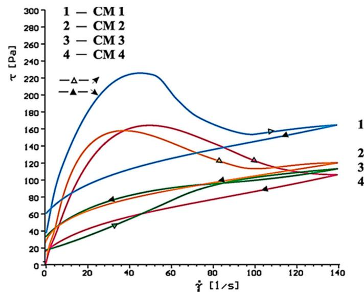
**Figure 15.** Flow curves of cementitious pastes containing 5% by mass of  $\text{CaSO}_4 \cdot 0.5\text{H}_2\text{O}$  and  $\text{CaSO}_4$  in quantity from 20 to 80% by mass, after 60 min.
