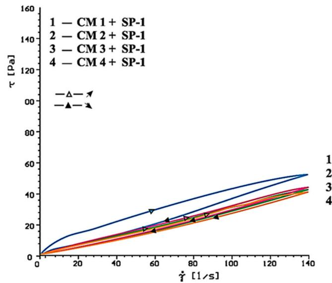
Figure 16. Flow curves of cementitious pastes containing 5% by mass of  $\text{CaSO}_4 \cdot 0.5\text{H}_2\text{O}$  and  $\text{CaSO}_4$  in quantity from 20 to 80% by mass in presence of SP-1 type superplasticizer, 1% by mass, after 10 min.
