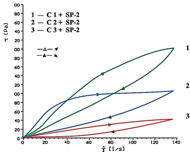
**Figure 11.** Flow curves of cement pastes with addition of  $\text{CaSO}_4 \cdot 0.5\text{H}_2\text{O}$ ,  $\text{CaSO}_4$ ,  $\text{CaSO}_4 \cdot 2\text{H}_2\text{O}$  in presence of SP-2 superplasticizer, after 60 min.
