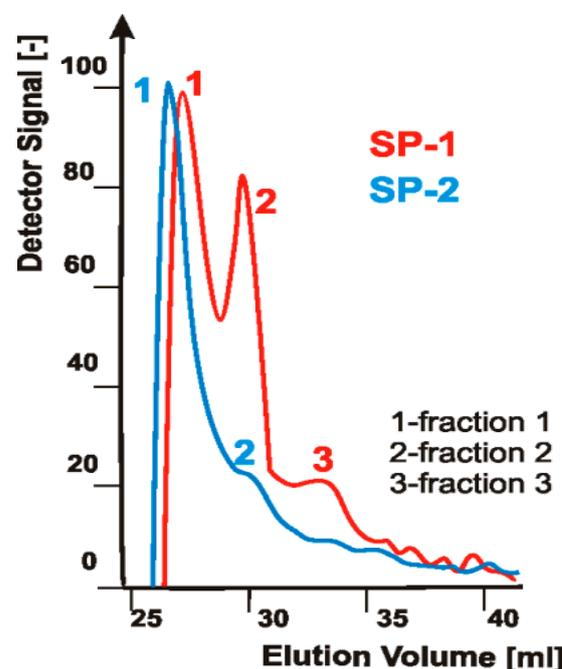
Figure 1. GPC chromatograms of superplasticizers specimens (SP-1, SP-2), [based on results published in [41]].
