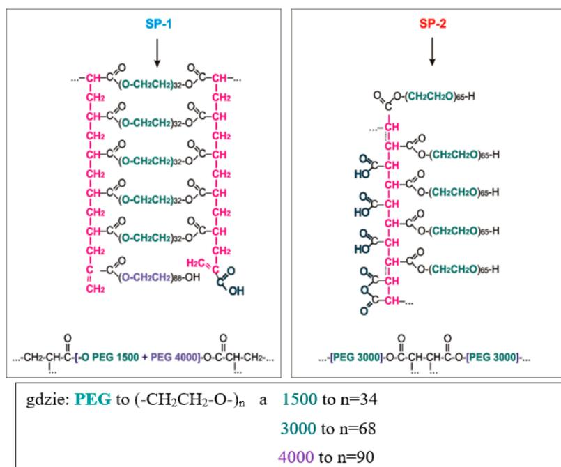
**Figure 4.** Approximate chemical structures of superplasticizers: ladder-shaped (SP-1) and comb-shaped (SP-2) determined based on mathematical calculation of molar masses.
