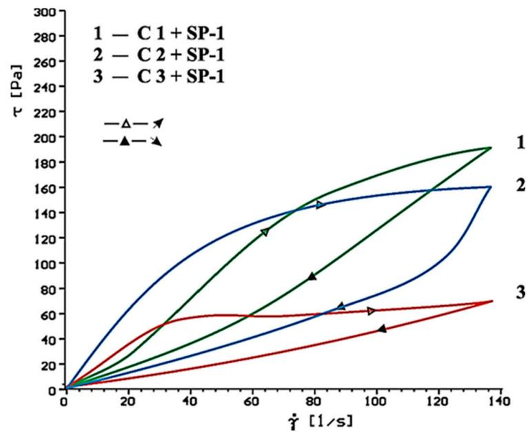
Figure 9. Flow curves of cement pastes with addition of  $\text{CaSO}_4 \cdot 0.5\text{H}_2\text{O}$ ,  $\text{CaSO}_4$ ,  $\text{CaSO}_4 \cdot 2\text{H}_2\text{O}$  in presence of SP-1 superplasticizer, after 60 min.
