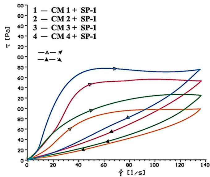
Figure 17. Flow curves of cement pastes containing 5% by mass of  $\text{CaSO}_4 \cdot 0.5\text{H}_2\text{O}$  and  $\text{CaSO}_4$  in quantity from 20 to 80% by mass in presence of SP-1 type superplasticizer, 1% by mass, after 60 min.
