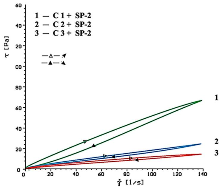
Figure 10. Flow curves of cement pastes with addition of  $\text{CaSO}_4 \cdot 0.5\text{H}_2\text{O}$ ,  $\text{CaSO}_4$ ,  $\text{CaSO}_4 \cdot 2\text{H}_2\text{O}$  in presence of SP-2 superplasticizer, after 10 min.
