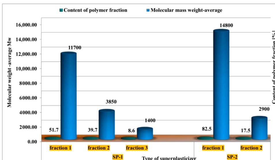
**Figure 2.** Results of the GPC chromatographic analysis of superplasticizer polymer fractions (SP-1, SP-2), [based on results published in [41]].
