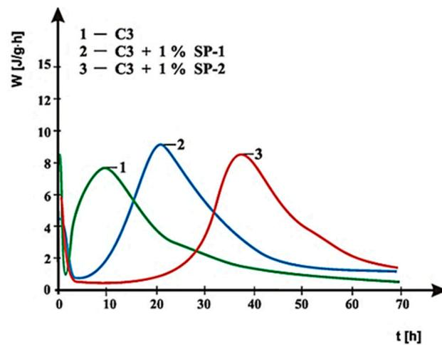
Figure 23. Hydration heat evolution rate curves for C3 cement without and with 1% by mass of SP-1 and SP-2 superplasticizers.
