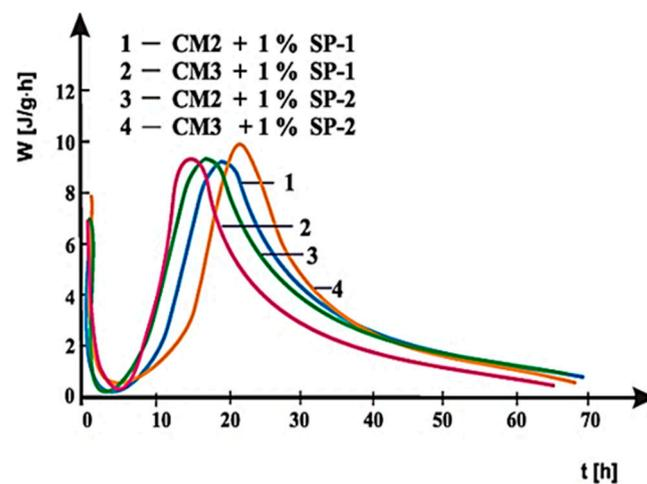
Figure 24. Hydration heat evolution rate curves for CM2 and CM3 cements with 1% by mass of SP-1 and SP-2 superplasticizers.
