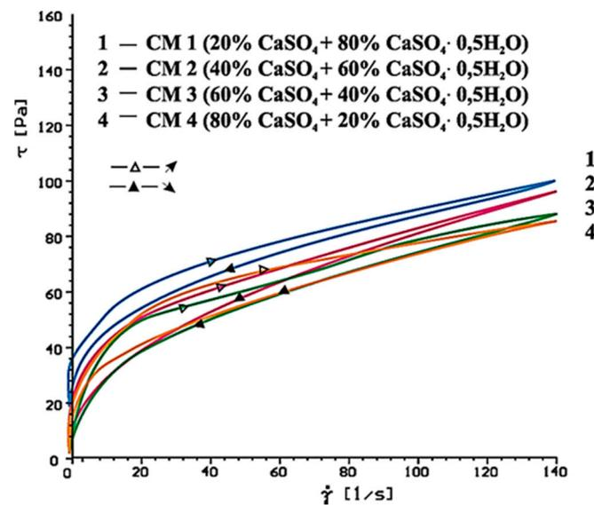
**Figure 14.** Flow curves of cementitious pastes containing 5% by mass of  $\text{CaSO}_4 \cdot 0.5\text{H}_2\text{O}$  and  $\text{CaSO}_4$  in quantity from 20 to 80% by mass, after 10 min.
