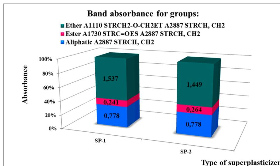
**Figure 5.** Results of FTIR spectral analysis of superplasticizer samples (based on results published in [41]).
