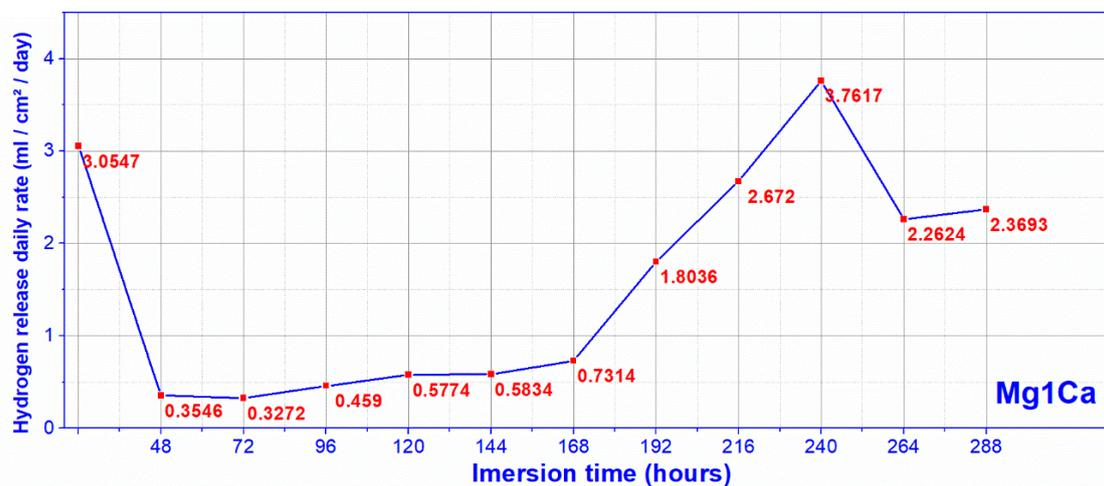
Figure 8. Hydrogen release rate, Dulbecco (mean values for three samples).
