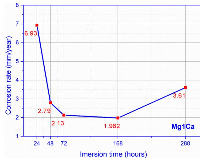
**Figure 9.** Corrosion rate, Dulbecco (mean values for three samples).
