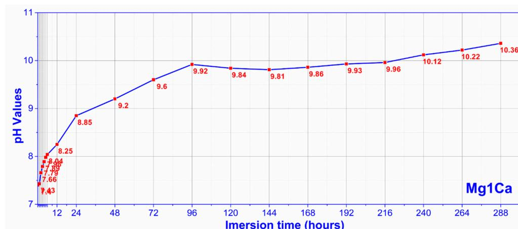
Figure 6. pH evolution in SBF (mean values for three samples).
