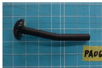
Figure 10. Failure mode of FRTTP rivet under bending.
