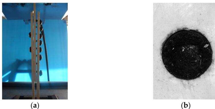
Figure 13. Typical failure mode. (a) Failure mode of eight-rivet specimen; (b) close-up image around FRTP rivet.
