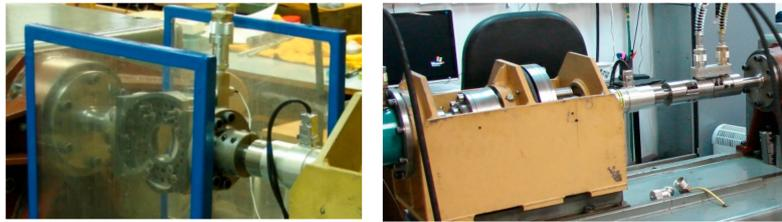
**Figure 4.** The load case of bending and pressurizing with the pressure chamber and the pressure sensor—FF046 load case (left). The setup of the test case with the pressure chamber inducing inner and outer pressure—FF059 load case (right).
