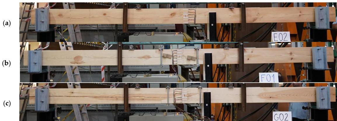
**Figure 11.** View of an example beam in each series: (a) series E—with 2 drawbolts (double-sided tooth plate connectors type C10 + M10 screws), (b) series F—with wood inserts (and additional steel clamps), (c) series G—with steel clamps.
