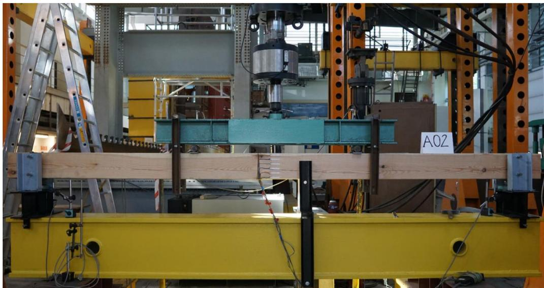
**Figure 14.** View of experimental stand for testing with an example beam.
