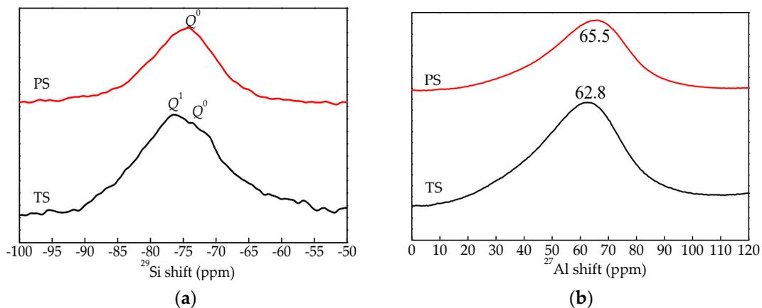
**Figure 6.**  $^{29}\text{Si}$  and  $^{27}\text{Al}$  NMR spectroscopy for two kinds of water-quenched slag. (a)  $^{29}\text{Si}$  NMR spectroscopy; (b)  $^{27}\text{Al}$  NMR spectroscopy.
