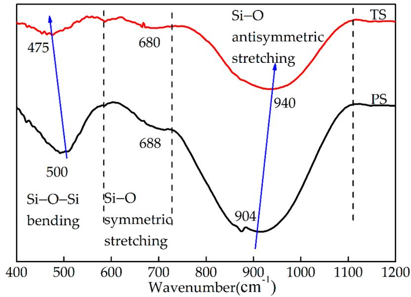
Figure 4. FTIR spectroscopy of two kinds of water-quenched slag.
