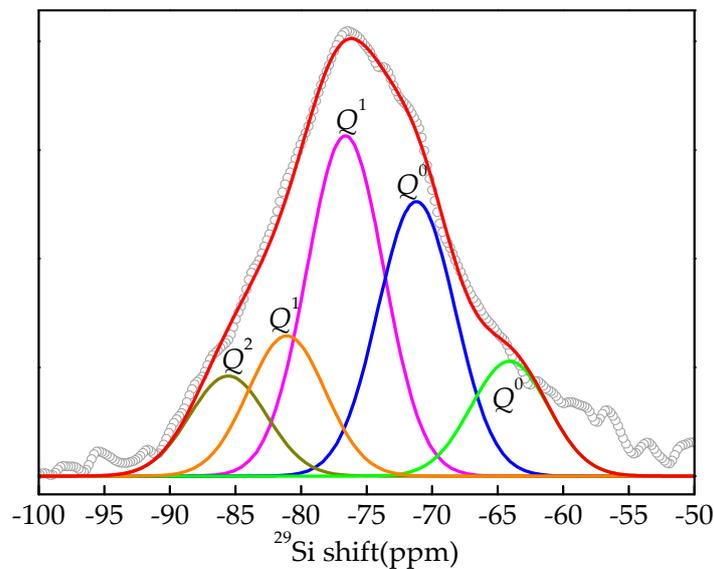
Figure 7. Deconvolution of  $^{29}\text{Si}$  NMR spectroscopy of water-quenched high-titanium slag.
