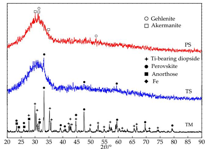
**Figure 1.** XRD patterns of three kinds of slag.
