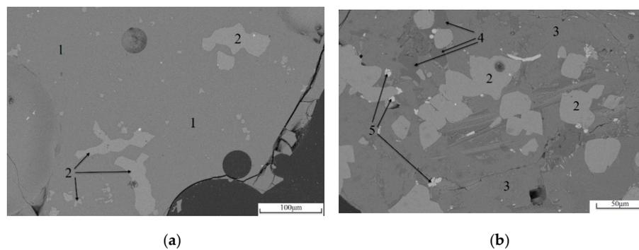
**Figure 2.** SEM images of two kinds of high-titanium slag. (a) TS; (b) TM.
