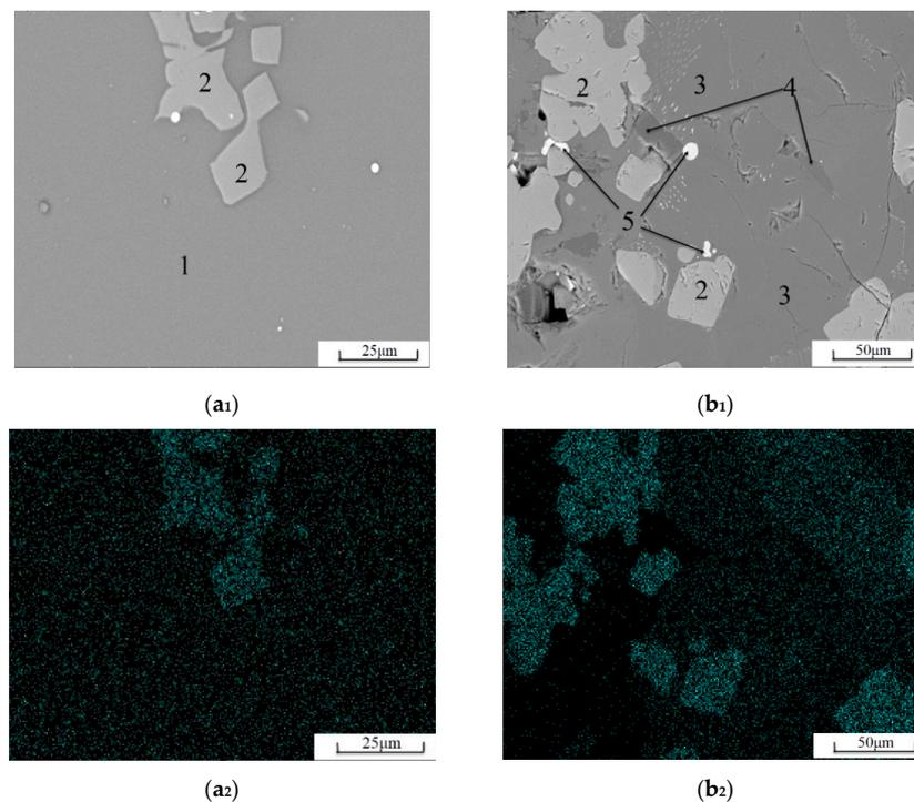
**Figure 3.** SEM images of Ti surface scanning of high-titanium slag. (a<sub>1</sub>) SEM image of TS; (a<sub>2</sub>) Ti surface scanning of TS; (b<sub>1</sub>) SEM image of TM; (b<sub>2</sub>) Ti surface scanning of TM.
