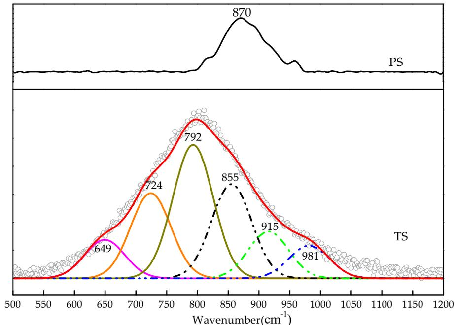
Figure 5. Raman spectroscopy of two kinds of water-quenched slag.
