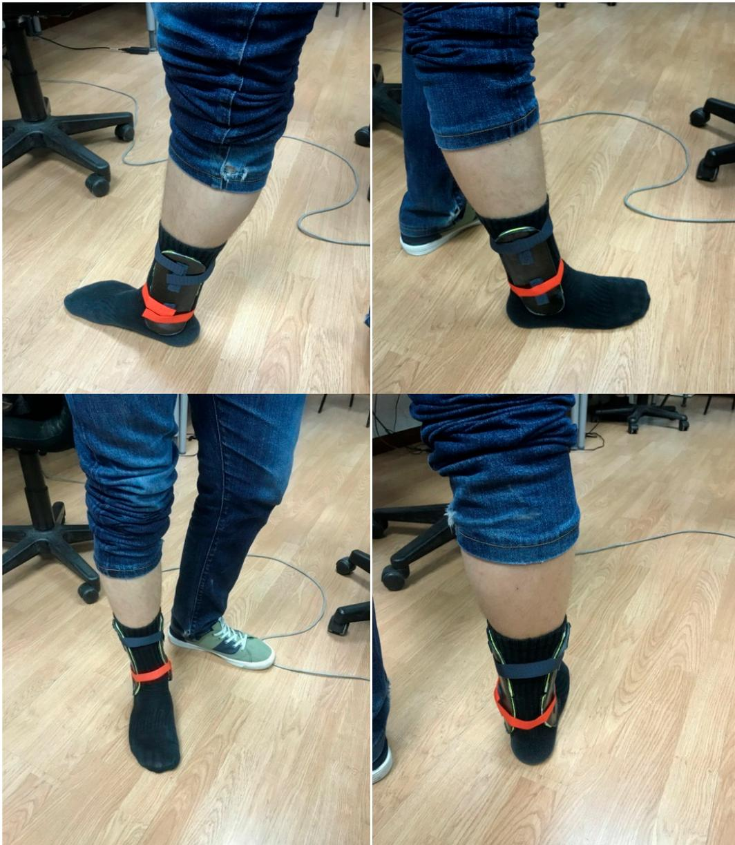
**Figure 7.** Evaluation of ergonomic performance upon healthy volunteer, after adding inner glued soft protective pads and fixation strips to the carbon fiber splint structures.
