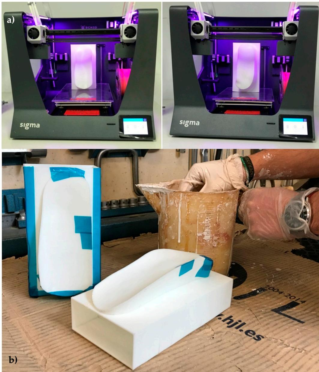
**Figure 3.** Rapid mold manufacture procedure by 3D printing and clay filling: Two molds are used for the double-sided ankle splint aimed at improved immobilization. (a) 3D printing. (b) Filling with clay.
