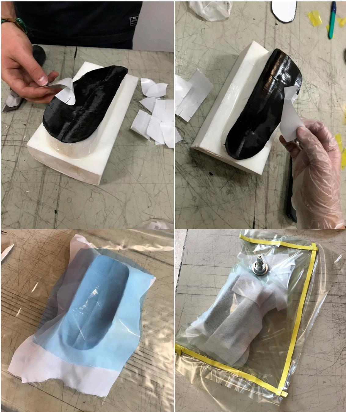
**Figure 4.** Lamination of composite fibers upon 3D-printed molds and pressurization during curing toward the final personalized orthoses.
