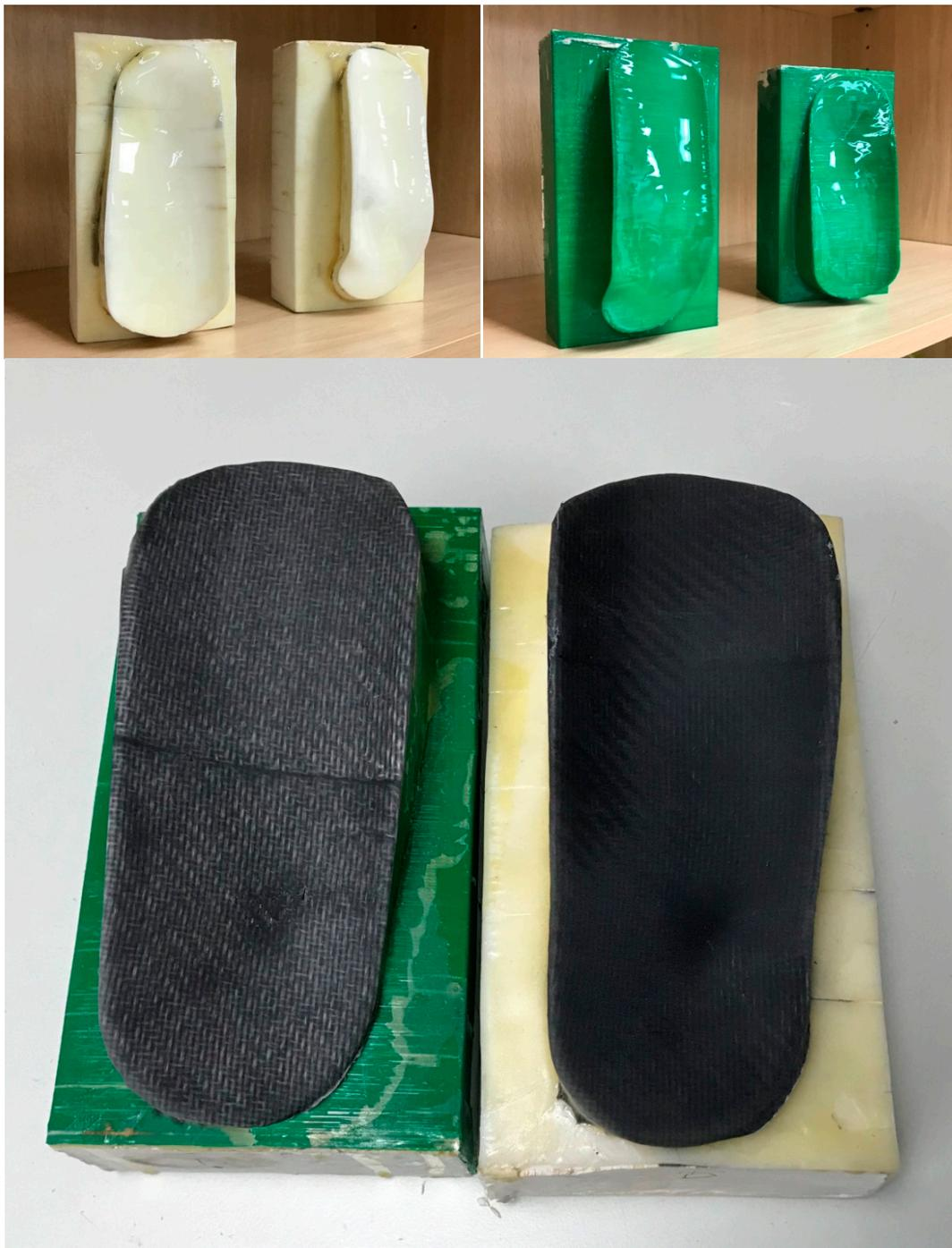
**Figure 6.** Final 3D-printed molds with the obtained personalized ankle splints in carbon fiber.
