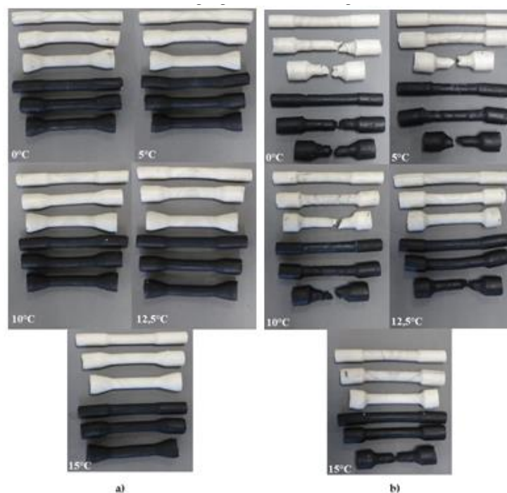
Figure 12. The forgings obtained in the processes of modelling: (a) slippages, neckings and ruptures (test 1); (b) inner defects (test 2).
