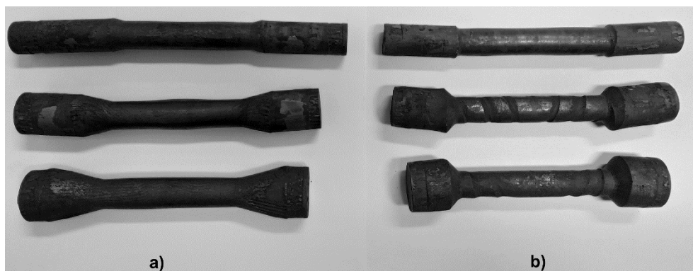
Figure 9. The elements obtained from laboratory testing of the real material using hot-formed 50HS steel: (a) test 1, (b) test 2.
