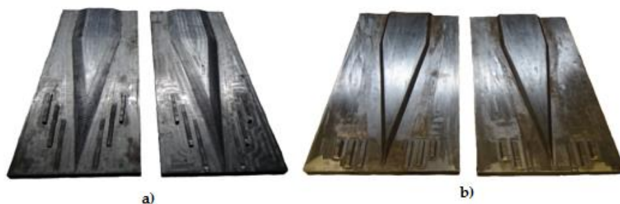
Figure 5. The tools used for testing the limits of cross-wedge rolling of 50HS grade steel in hot working conditions: (a) inner cracks (Test 1); (b) slippages, neckings and ruptures (Test 2).
