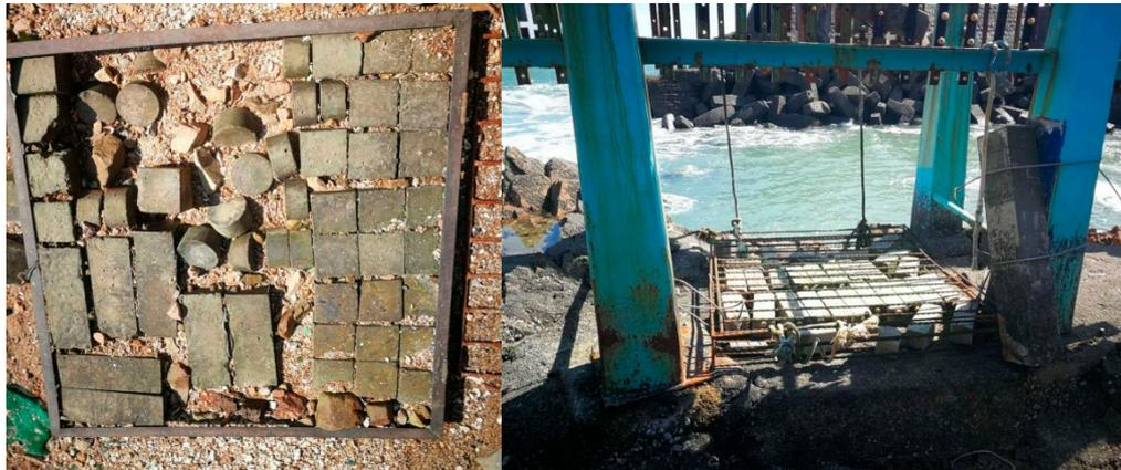
**Figure 3.** Architectural concrete exposed to actual marine environments.
