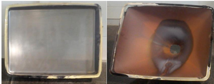
**Figure 1.** Left, front part cathode ray tube (CRT<sub>F</sub>); right, rear part (CRT<sub>R</sub>).
