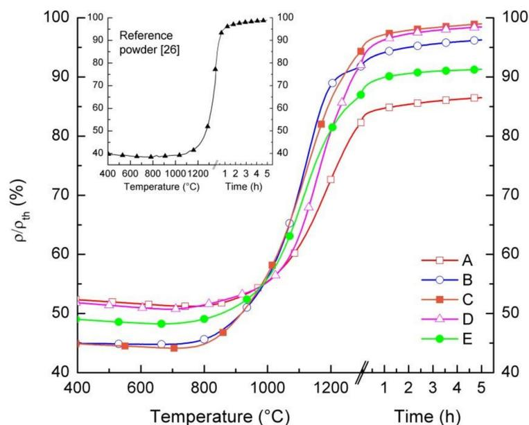
**Figure 4.** Relative density of pressed pellets prepared by the five LSCF powders as a function of temperature and dwell time. The inset shows the relative density of a pellet prepared by the reference powder, up to a temperature of  $1350\text{ }^\circ\text{C}$  with a dwell time of 5 h.
