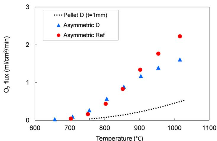
**Figure 13.** Oxygen flux as a function of the temperature. Results of permeation tests performed on an asymmetric membrane manufactured with the reference powder and on a pellet and an asymmetric membrane manufactured with the Praxair powder (D) selected in this work.
