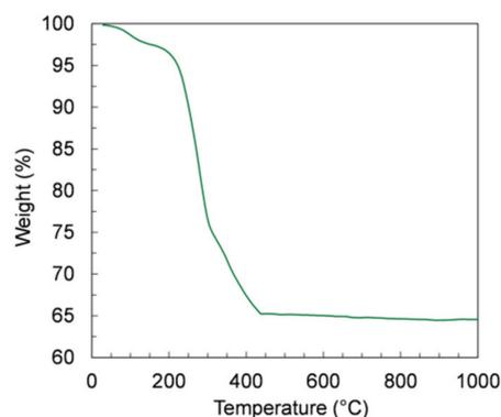
**Figure 9.** Thermogravimetric analysis (TGA) curve of the green tape prepared using powder D and *slurry 4*.
