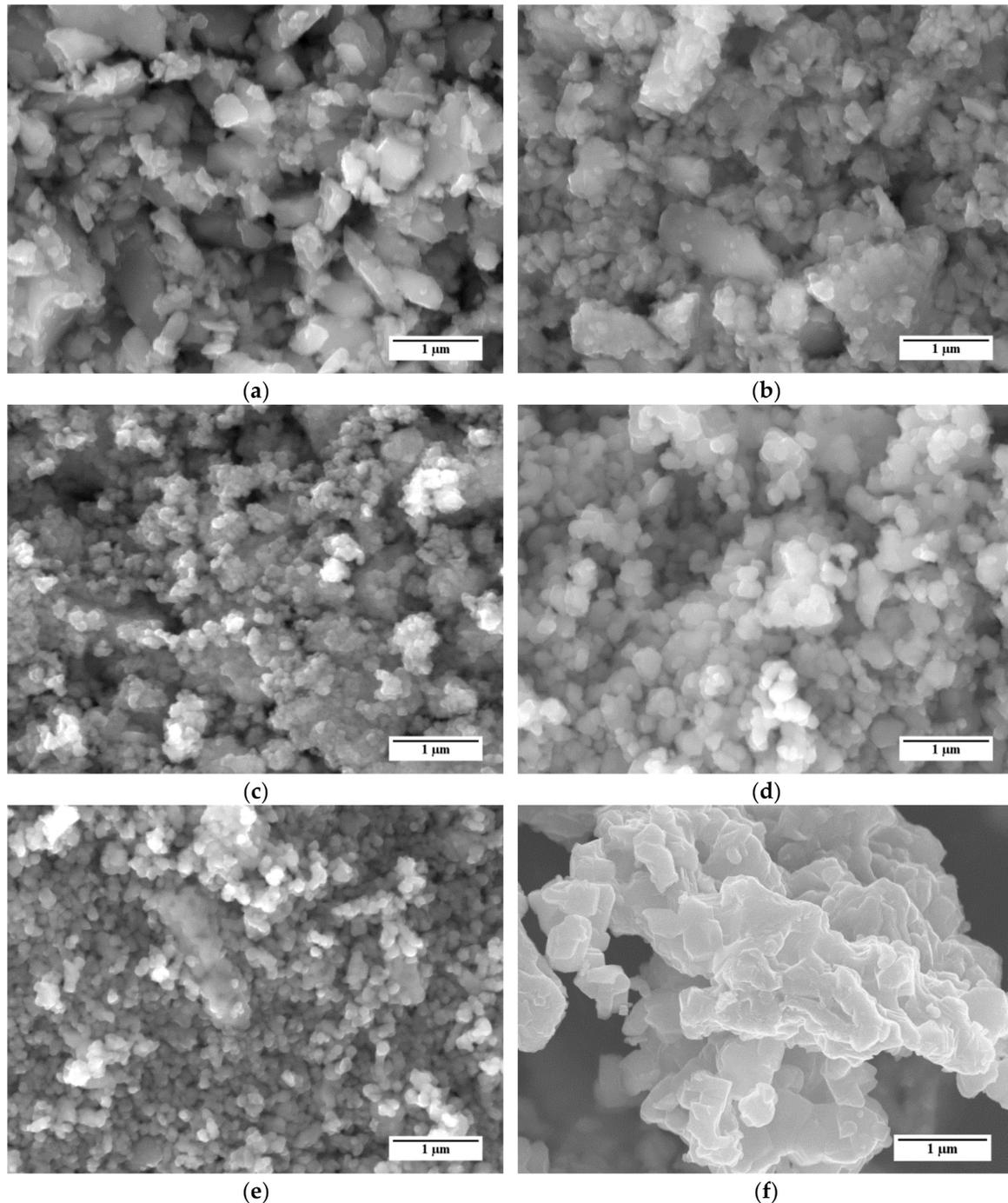
**Figure 2.** SEM micrographs of the  $\text{La}_{0.6}\text{Sr}_{0.4}\text{Co}_{0.2}\text{Fe}_{0.8}\text{O}_{3-\delta}$  (LSCF) powders considered in this study: (a) Powder A; (b) Powder B; (c) Powder C; (d) Powder D; (e) Powder E; (f) Reference powder.
