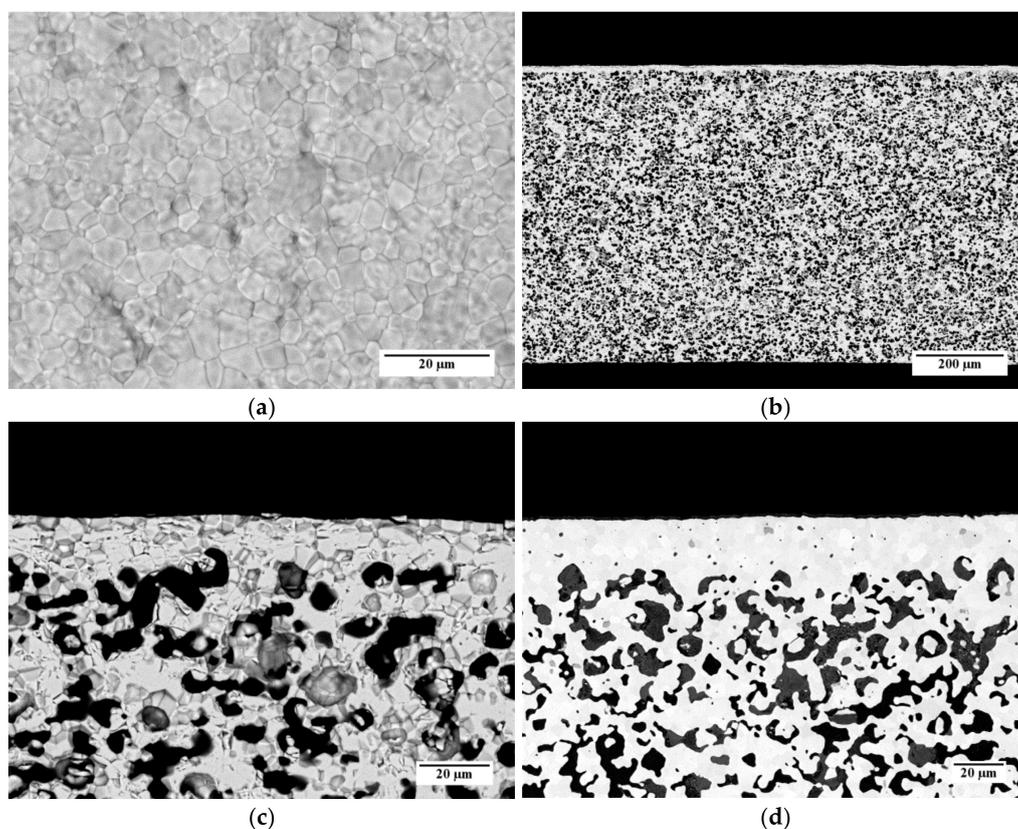
**Figure 11.** SEM micrographs of a membrane obtained using powder D from *slurry 3* and sintered by *TT3*: (a) Aspect of the membrane layer surface; (b) Cross-section; (c) Detail of the cross-section; (d) Detail of the cross-section of a membrane realized by the reference powder and recipe.
