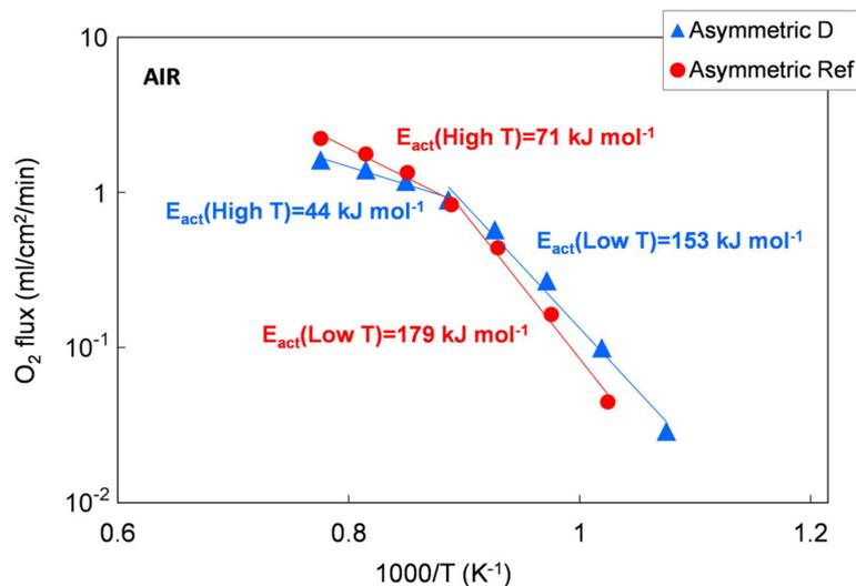
**Figure 14.** Oxygen flux as a function of temperature. Results of permeation tests performed on a membrane manufacture with the reference powder and with the Praxair powder (D) selected in this work.
