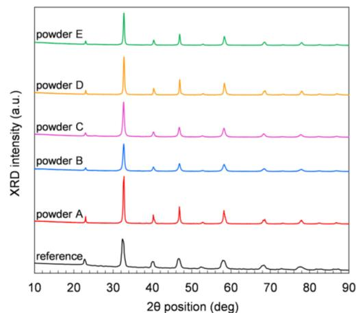
**Figure 3.** XRD patterns of the LSCF powders measured at room temperature.
