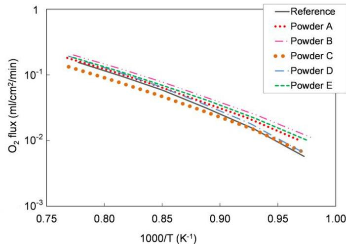
**Figure 5.** Oxygen flux normalized with respect to the process driving force as a function of temperature measured for pellets prepared with the five different LSCF powders, compared with that measured for a reference LSCF powder pellet. Samples thickness = 1 mm. Experimental error approx. 5%.
