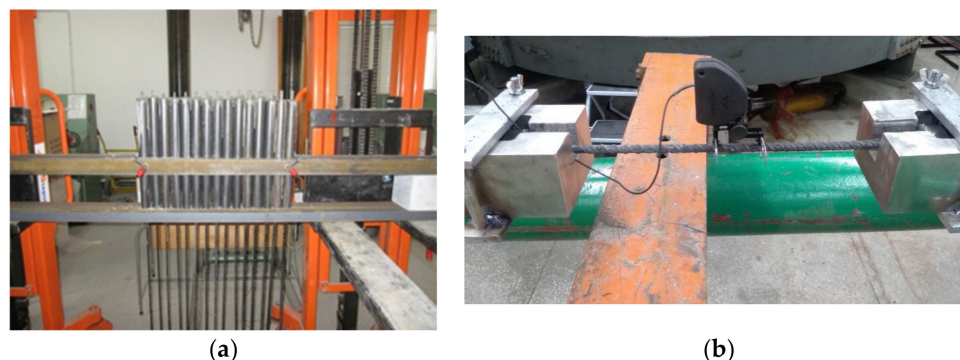
Figure 2. (a) Basalt Fiber Reinforced Polymers (BFRP) bars prepared for testing, (b) Hybrid Fiber Reinforced Polymers (HFRP) bars in the tensile testing machine.
