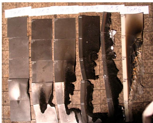
**Figure 18.** Test samples TGM 1 to TGM 6 after carrying out the Schlyter test. (TGM1: PP + 5%Gra, TGM2: PP + 5%Gra + 5%AlPh, TGM3: PP + 5%Gra + 5%MMT, TGM4: PP + 5%Gra + 5%AlPh + 5%MMT, TGM5: PP + 5%Gra + 5%MgOH, TGM6: PP + 5%MgOH).
