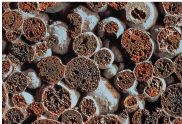
**Figure S4.** The fracture surface of the commercially available Liapor aggregate.
