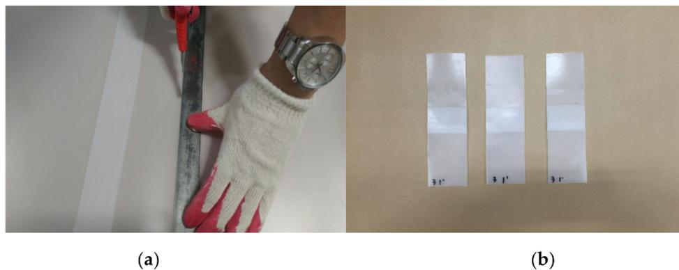
**Figure 4.** Joint hot air welding construction status: (a) specimen fabrication status; and (b) a joint tensile performance test specimen.
