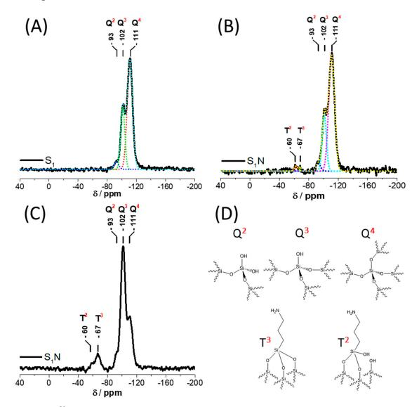
**Figure 2.** <sup>29</sup>Si MAS NMR spectra of (**A**) S<sub>1</sub> and (**B**) S<sub>1</sub>N; the dashed lines represent deconvoluted curves obtained by using a Gaussian function. (**C**) <sup>29</sup>Si {<sup>1</sup>H} CP/MAS NMR spectrum of S<sub>1</sub>N. (**D**) Illustration of Q<sup>2, 3, 4</sup> and T<sup>2, 3</sup> groups.
