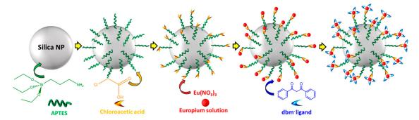
Scheme 1. Scheme illustrating the sequence of reaction steps for the luminescent hybrid production.
