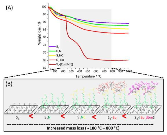
**Figure 3.** (**A**) Thermogravimetric curves of all samples obtained after each functionalization step. (**B**) Surface illustrative representation of all samples, elucidating the increase of organic matter losses during the second thermal event.
