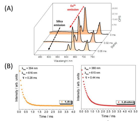
**Figure 6.** (**A**) Time-resolved emission spectra of S<sub>1</sub>-[Eu] with  $\lambda_{ex} = 394$  nm; (**B**)  ${}^{5}D_{0}$  excited state decay curves of S<sub>1</sub>-[Eu] and S<sub>1</sub>-[Eu(dbm)].
