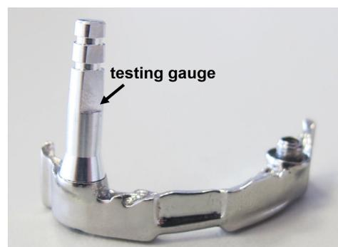
Figure 7. Dental framework with testing gauge.
