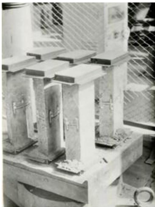
Figure 4. Prism specimens prepared for testing.
