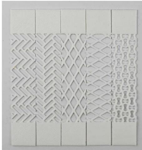
**Figure 6.** 3D printed pattern-specimens of TPU 95A.
