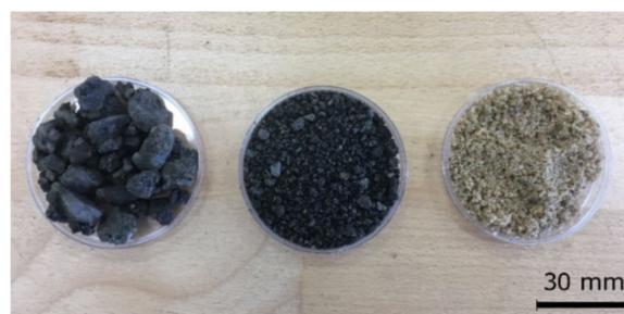
**Figure 1.** Samples of silica aggregate and RAP aggregate after separation of coarse particles.
