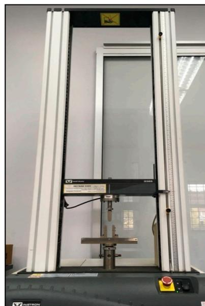
**Figure 6.** Flexural test setup using an Instron universal testing machine model 3365.
