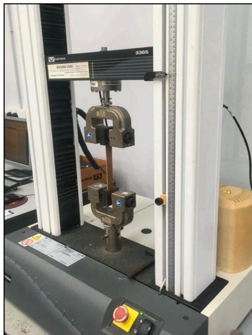
**Figure 4.** Tensile test setup using an Instron universal testing machine model 3365.
