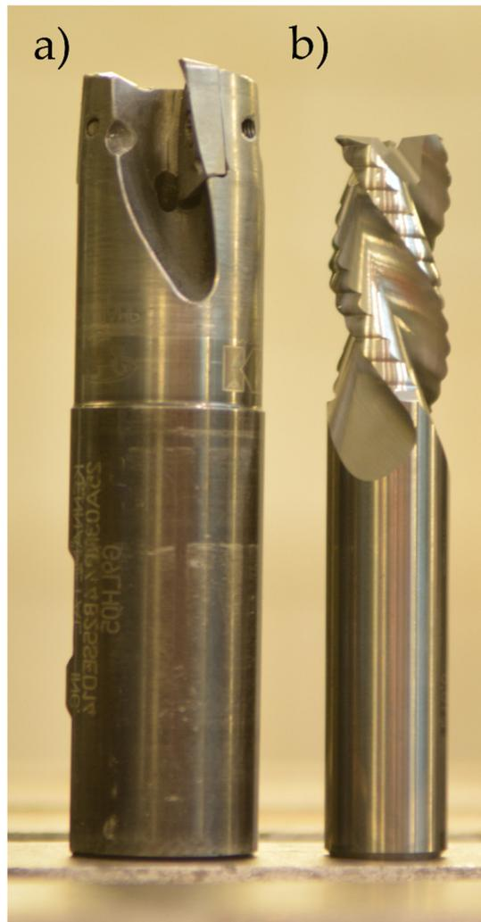
**Figure 4.** Tools used: (a) Kennametal indexable milling cutter, (b) Sandvik monolithic milling cutter.
