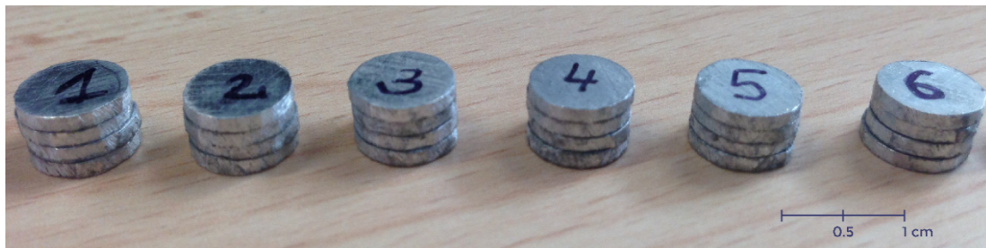
Figure 5. Split Hopkinson pressure bar (SHPB) specimen's built using four disks cut from the aluminum sheet of 1 mm thickness.
