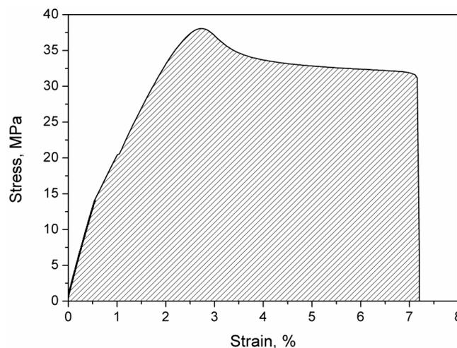
**Figure 4.** Exemplary stress–strain curve for the 1W45 sample.
