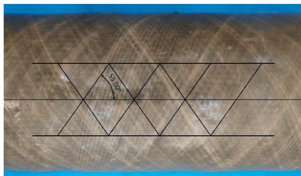
Figure 1. Alignment of fibers in filament-wound pipes.
