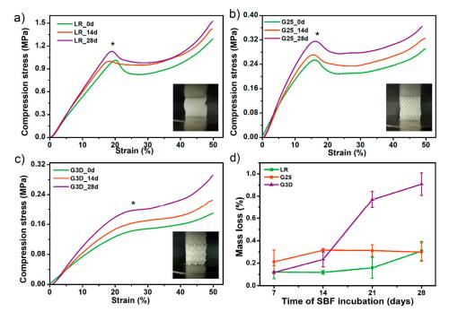
Figure 10. The influence of incubation in simulated body fluid SBF solution on compressive strength (a-c) and mass loss (d) of selected porous tissue structures PTS. \* The inflexion point of the stress-strain curves (the so-called Yield point) was assumed as the compressive strength values of studied PTS.
