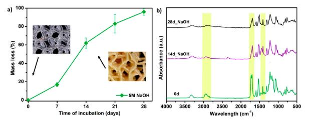
**Figure 11.** The results of accelerated degradation studies on G25 PTS in 5 M sodium hydroxide NaOH, (a) mass loss measurements, (b) FTIR spectra. SEM images showing the accelerated degradation process are presented in supplementary data (Table S7).
