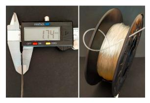
Figure 2. View of obtained TPU\_F filament.
