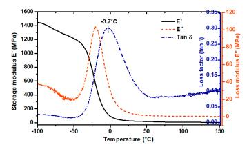
**Figure 6.** Dynamic mechanical analysis DMA results of TPU printout. Storage modulus (E'), loss modulus (E'), loss factor (Tan  $\delta$ ).
