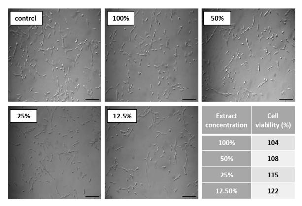
**Figure 8.** Results of cytotoxicity test. Images show CCL-163 cells morphology after 24 h contact with TPU\_P extracts of specified concentrations (100–12.5%). Scale bar =  $50 \mu m$ . The table present percentage of cell viability towards control (100%). SD were negligibly small, there were no statistical differences between the obtained results.
