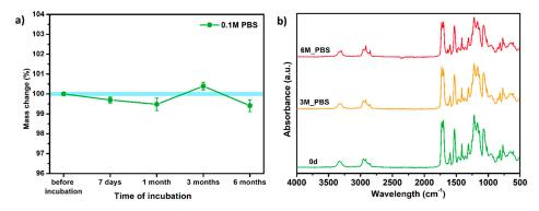
**Figure 7.** The results of long-term degradation studies on TPU\_P samples in  $0.1 \, \text{M}$  phosphate-buffered saline PBS solution (37 °C), (a) mass change measurements, (b) FTIR spectra. Optical images can be found in supplementary data Table S6.
