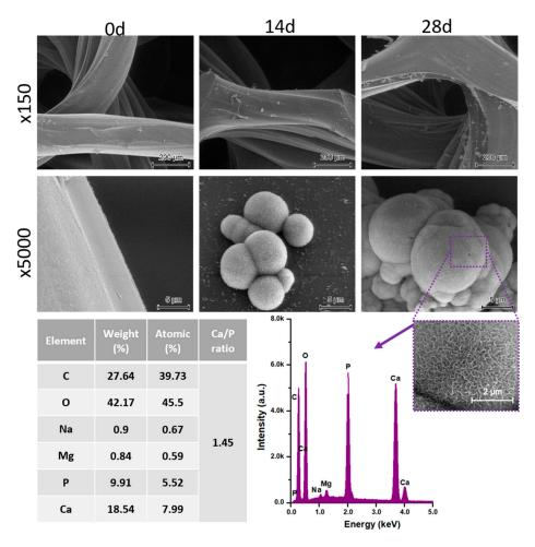
Figure 9. SEM images and EDS spectrum of G25 PTS after incubation in SBF.
