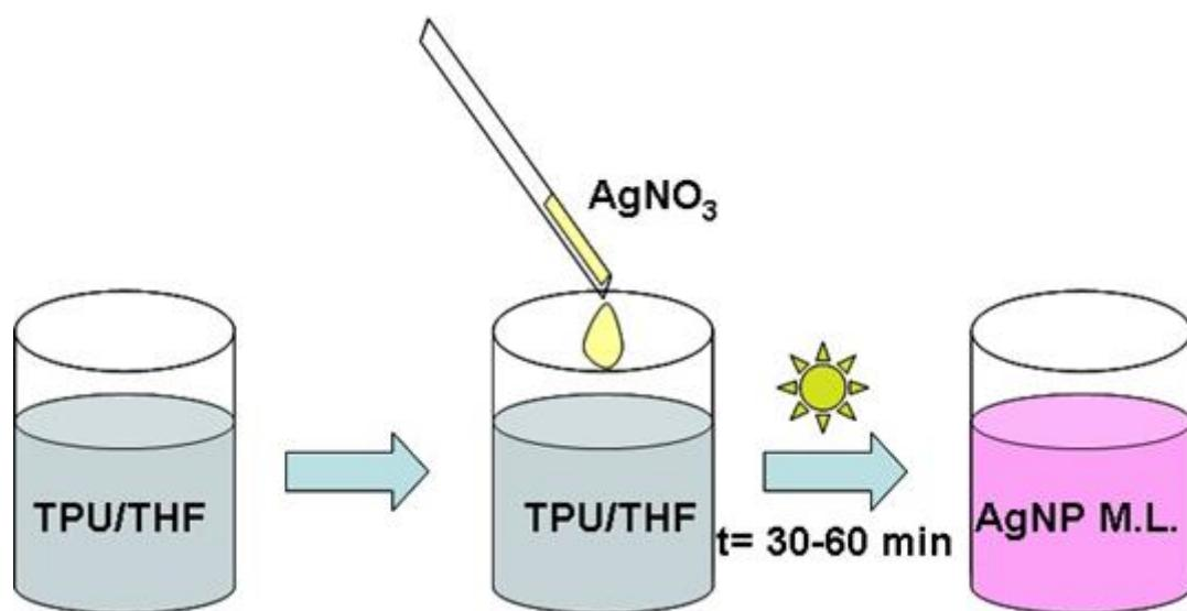
**Figure S1.** Schematic representation of the general procedure used for the preparation of M.L.
