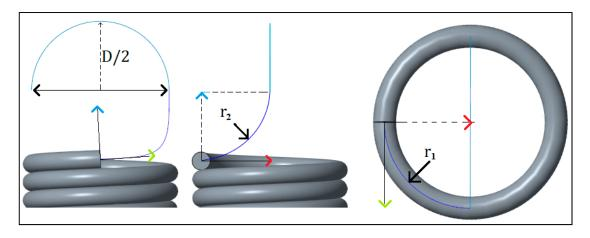
Figure 5. CAD modeling parameters for hook's arc.
