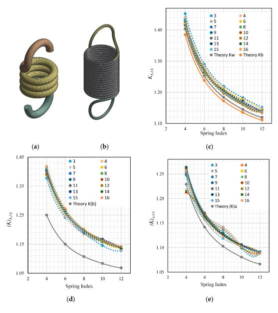
**Figure 10.** Change of parameter from (**a**) N = 3, C = 4 to (**b**) N = 16, C = 12; effects of spring index and number of coils against (**c**)  $K_{b,FE}$ , (**d**)  $(K)_{b,FE}$ , (**e**)  $(K)_{a,FE}$ .
