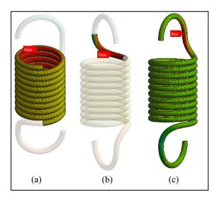
Figure 8. Locations of maximum stress in (a) the body, (b) point B and (c) point A.
