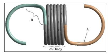
Figure 2. Extension spring critical points.
