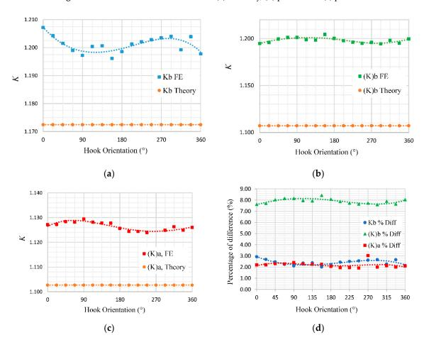
**Figure 9.** Effect of hook orientation on  $K_{FE}$  measured at (a) the spring body, (b) point B and (c) point A; (d) the percentage of difference between the correction factors obtained through the FE methods and the theoretical approach.
