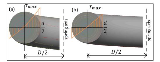
Figure 1. The effect of spring index toward distribution of stress: (a) small index, (b) large index.
