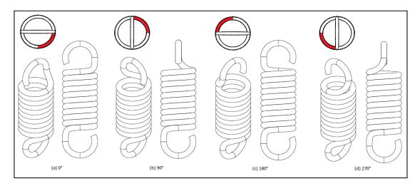
**Figure 3.** Hook orientations with varying degrees of offset (a)  $0^{\circ}$ , (b)  $90^{\circ}$ , (c)  $180^{\circ}$ , and (d)  $270^{\circ}$ ; the bottom hook was taken as reference.
