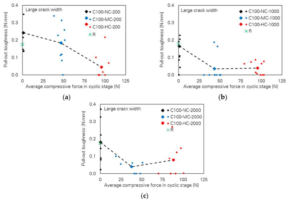
**Figure 6.** Influence of cyclic compressive force level on pull-out toughness of the specimens with large crack width; number of cycles: (a) 200, (b) 1000 and (c) 2000.
