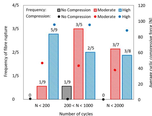
**Figure 9.** Frequency of fibre rupture during the cyclic stage depending on the number of cycles and compressive force on the fracture section.
