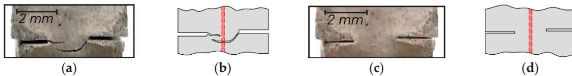
Figure 12. (a,b) Fracture pattern on the notch at the upper reversal point, (c,d) the deformed shape of the specimen at the lower reversal point.
