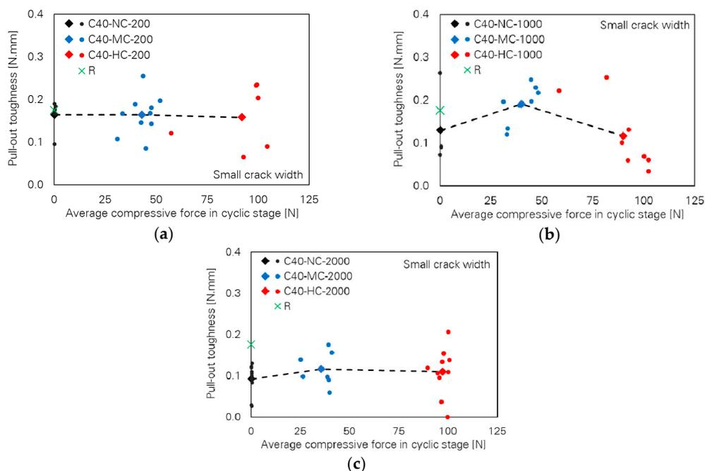
**Figure 3.** Influence of cyclic compressive force level on pull-out toughness of the specimens with small crack width; number of cycles: (a) 200, (b) 1000 and (c) 2000.
