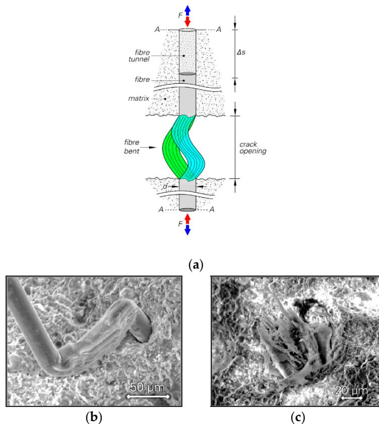
**Figure 11.** (a) Fibre bent due to large crack width under alternating tension–compression loading; scanning electron microscope (SEM) images reveal (b) the form of damage for C100-NC-2000-05 and (c) ruptured section of the fibre for C100-HC-1000-09.
