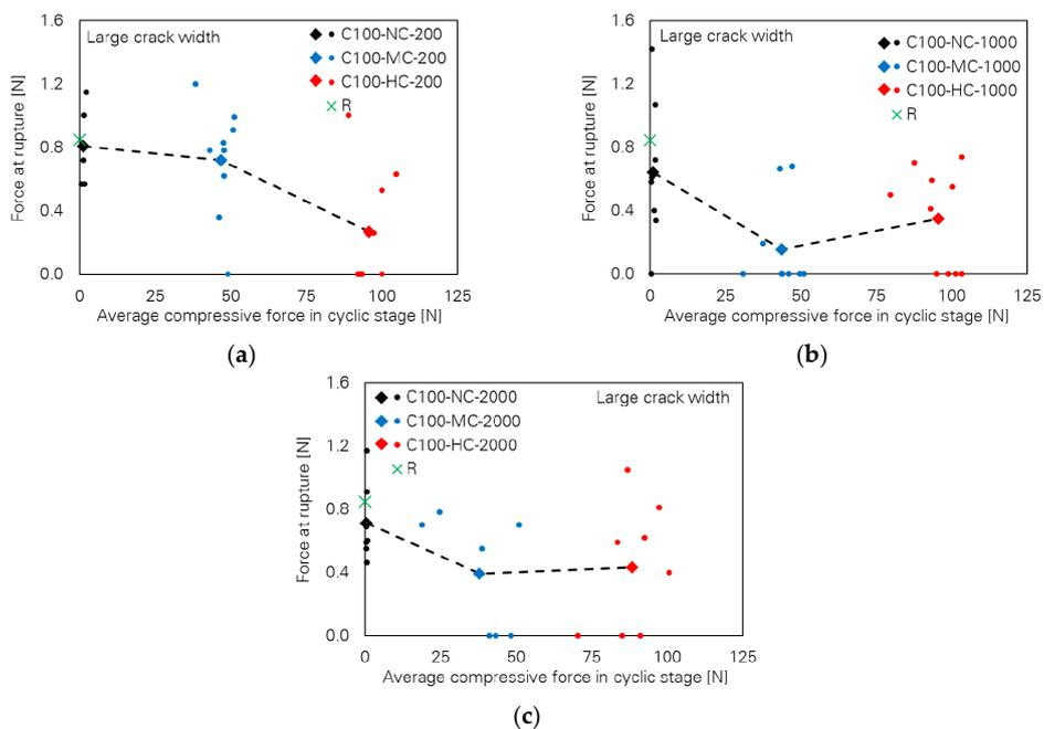
**Figure 7.** Influence of cyclic compressive force level on force at rupture of the specimens with large crack width; number of cycles: (a) 200, (b) 1000 and (c) 2000.
