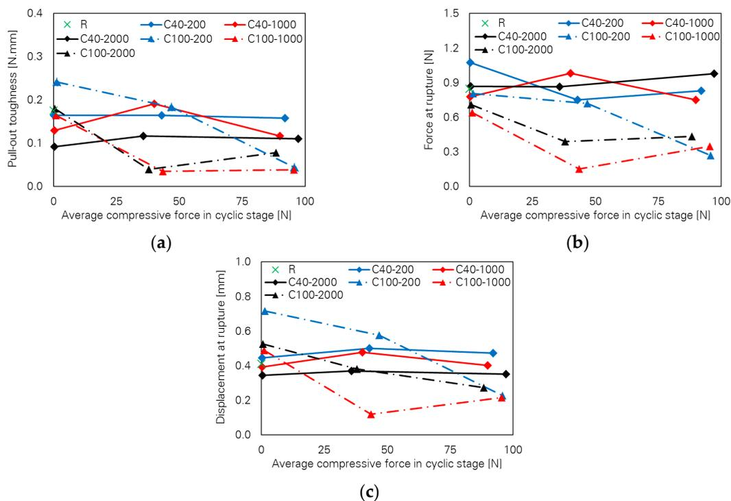
**Figure 10.** Combined influence of crack width and loading parameters on the crack-bridging capacity of PVA fibres: (a) pull-out toughness, (b) force and (c) displacement at fibre rupture.
