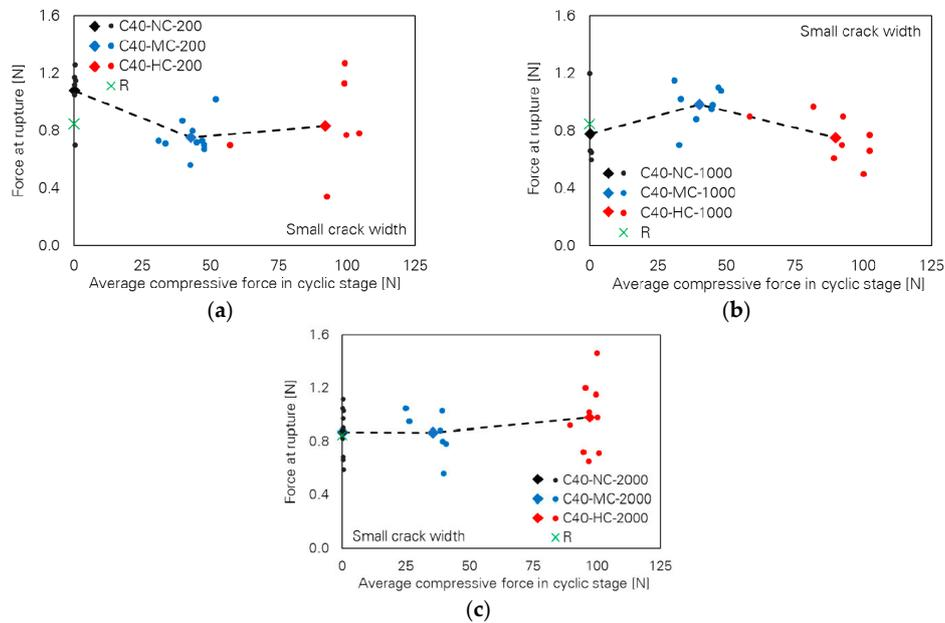
**Figure 4.** Influence of cyclic compressive force level on force at rupture of the specimens with small crack width; number of cycles: (a) 200, (b) 1000 and (c) 2000.
