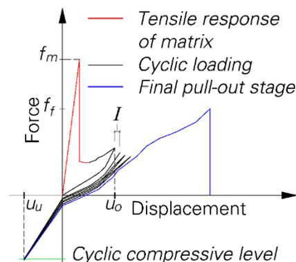
**Figure 2.** Progression of the force-displacement curve during different loading stages.
