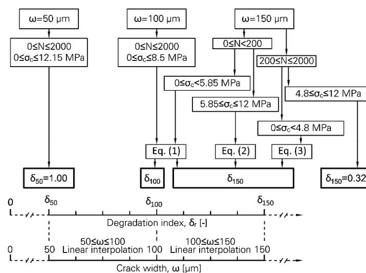
Figure 13. Suggested algorithm for estimation of the crack-bridging capacity of PVA microfibre and its degradation under alternating cyclic loading and under consideration of crack width.
