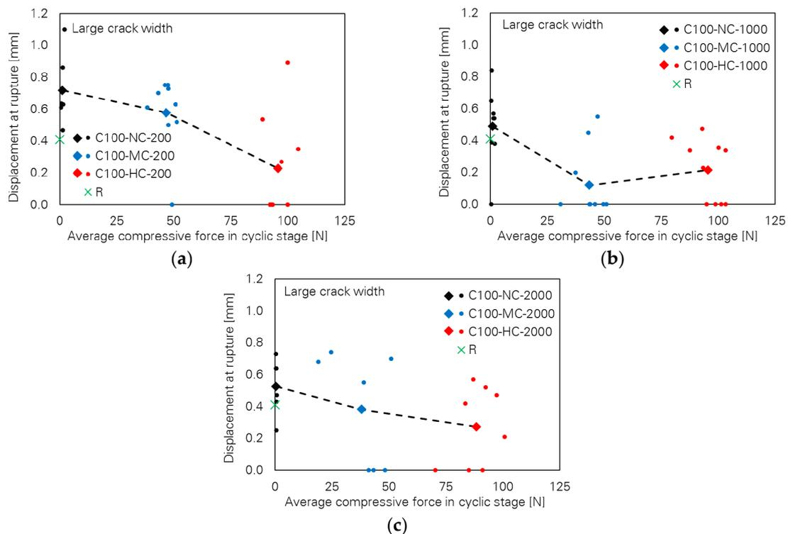
**Figure 8.** Influence of cyclic compressive force level on fibre displacement at rupture of the specimens with large crack width; number of cycles: (a) 200, (b) 1000 and (c) 2000.
