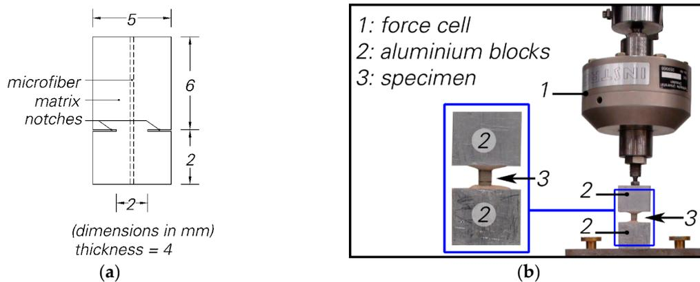
**Figure 1.** (a) The geometry of double-sided, single-fibre pull-out specimen, (b) the test setup configuration for double-sided, single fibre pull-out tests.
