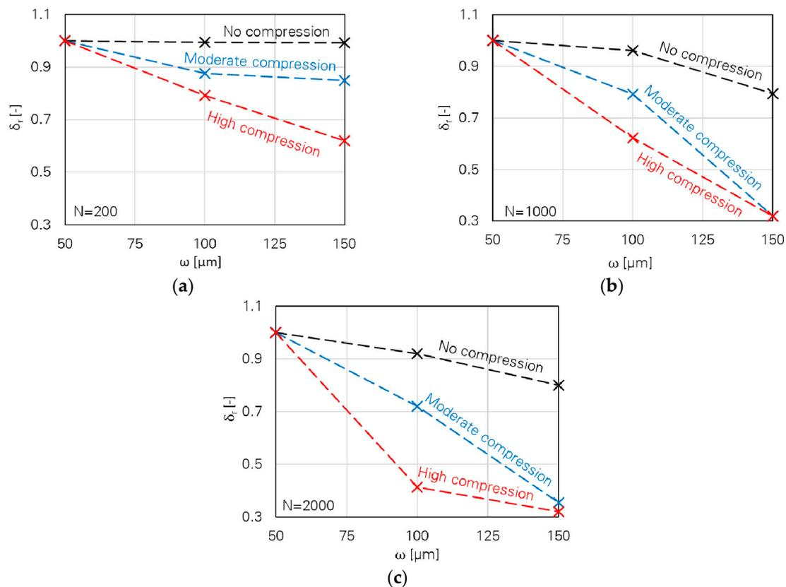
**Figure 14.** Degradation index ( $\delta_r$ ) as a function of crack width ( $\omega$ ), cyclic compressive stress ( $\sigma_c$ ) on the fracture surface, and number of cycles ( $N$ ): (a)  $N = 200$ , (b)  $N = 1000$  and (c)  $N = 2000$ .
