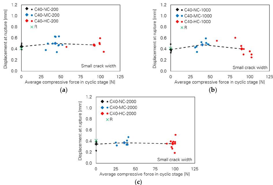
**Figure 5.** Influence of cyclic compressive force level on fibre displacement at rupture of the specimens with small crack width; number of cycles: (a) 200, (b) 1000 and (c) 2000.
