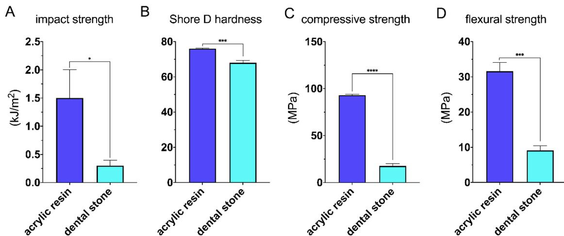
**Figure 4.** Mechanical properties of acrylic and plaster samples: (A) impact strength, (B) Shore D hardness, (C) compressive strength, and (D) flexural strength.
