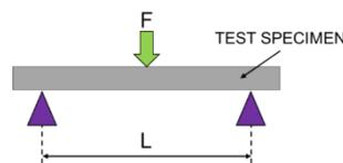
Figure 1. Schematic setup utilized for three-point bending test.
