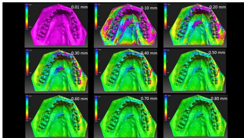
**Figure 2.** Maps of deviations prepared in accordance with the level of tolerance between 0.01 and 0.80 mm for sample number 1. Figure shows upon view areas where deviations are higher than the assumed level of tolerance as pink. Analysis was performed in three-dimensional perspective and the 0.80 mm level of tolerance was the lowest level without a deviation and are without pink areas.
