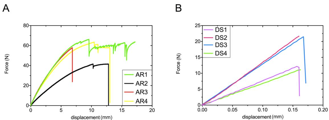
**Figure 5.** The force/displacement curves of acrylic (A) and stone samples (B) obtained during flexural strength evaluation. AR and DS means acrylic resin and dental stone, respectively (1–4 are the numbers of tested specimens).
