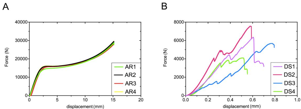
**Figure 6.** The force/displacement curves of acrylic (A) and stone samples (B) obtained during static compression test. AR and DS means acrylic resin and dental stone, respectively (1–4 are the numbers of tested specimens).
