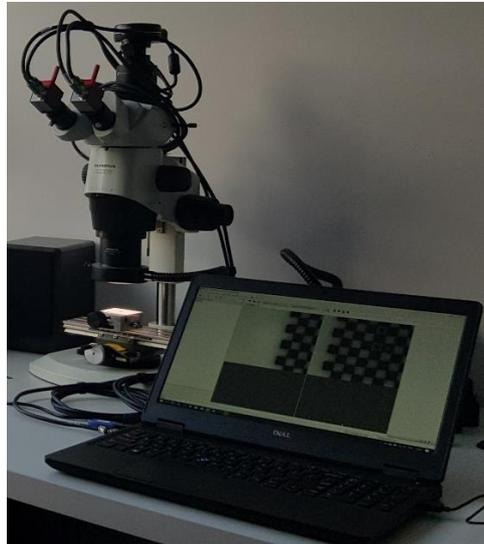
**Figure 2.** Equipment used for capturing the images of the tested specimen, and DIC analysis.
