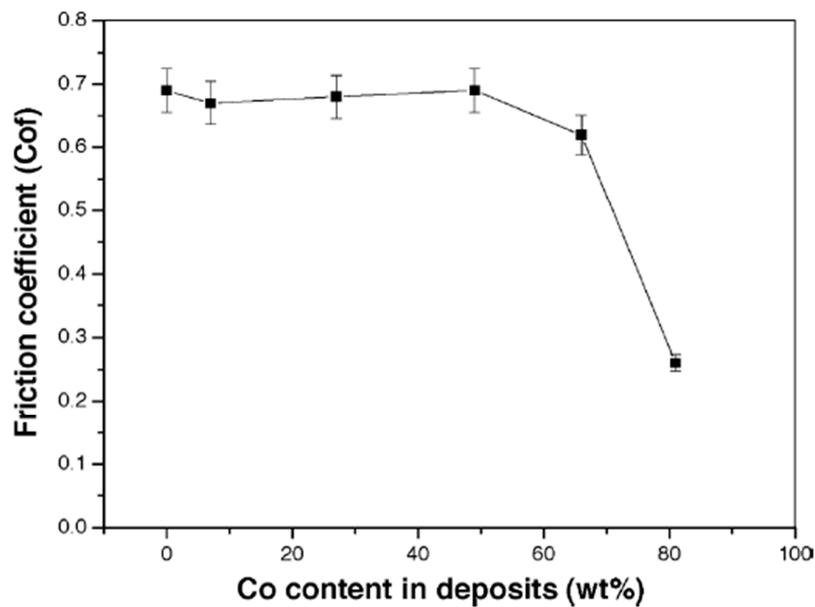
**Figure 11.** Friction coefficient as function of Co content in the Ni-Co alloy deposit [20]. Reprinted from Applied Surface Science, 242, Liping Wang, Yan Gao, Qunji Xue, Huiwen Liu, Tao Xu, Microstructure and tribological properties of electrodeposited Ni-Co alloy deposits/Pages No. 326–332, Copyright (2020), with permission from Elsevier.
