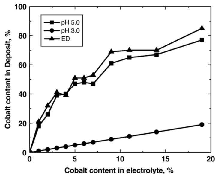
**Figure 6.** Alloy composition as a function of  $\text{Co}^{2+}$  concentration in the electrolyte [16]. Reprinted from Surface and Coatings Technology, 201, Meenu Srivastava, V. Ezhil Selvi, V.K. William Grips, K.S. Rajam, Corrosion resistance and microstructure of electrodeposited nickel-cobalt alloy coatings/Pages No. 3051–3060, Copyright (2020), with permission from Elsevier.
