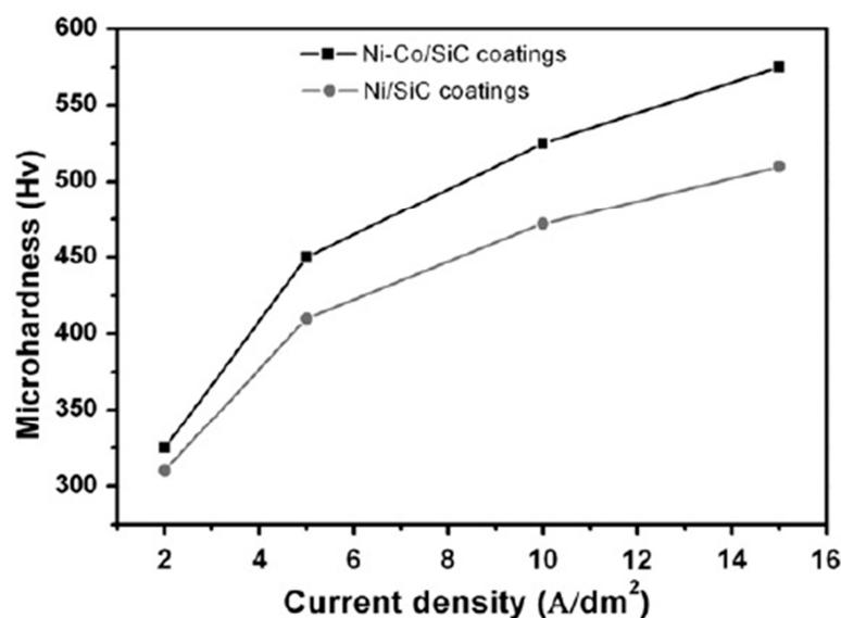
**Figure 9.** The effect of current density on microhardness of Ni–Co/SiC and Ni/SiC coatings [115]. Reprinted from *Surface and Coatings Technology*, 206, S.M. Lari Baghal, M. Heydarzadeh Sohi, A. Amadeh, A functionally gradient nano-Ni–Co/SiC composite coating on aluminum and its tribological properties/Pages No. 4032–4039, Copyright (2020), with permission from Elsevier.
