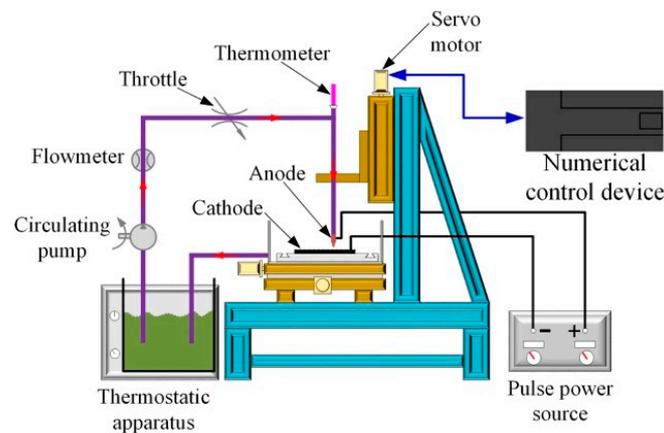
**Figure 1.** Schematic image of pulse jet electrodeposition.
