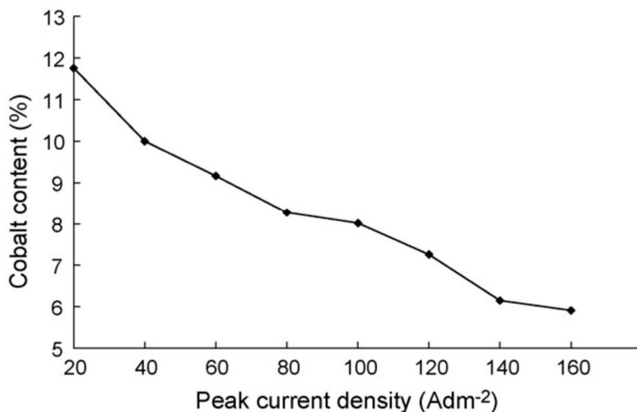
**Figure 3.** Cobalt content in Ni–Co alloy coatings with varying peak current density [34]. Reprinted from Applied Surface Science, 254, Yundong Li, Hui Jiang, Weihua Huang, Hui Tian, Effects of peak current density on the mechanical properties of nanocrystalline Ni–Co alloys produced by pulse electrodeposition/Pages No. 6865–6869, Copyright (2020), with permission from Elsevier.
