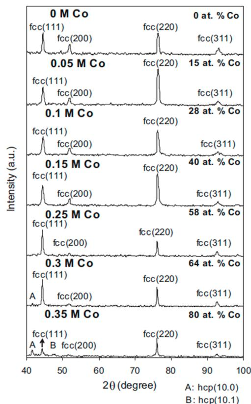
**Figure 7.** X-ray diffraction (XRD) patterns of Ni–Co films deposited from the electrolytes containing different Co concentrations [68]. Reprinted from Applied Surface Science, 258, Ali Karpuz, Hakan Kockar, Mursel Alper, Ozgur Karaagac, Murside Haciismailoglu, Electrodeposited Ni–Co films from electrolytes with different Co contents/Pages No. 4005–4010, Copyright (2020), with permission from Elsevier.
