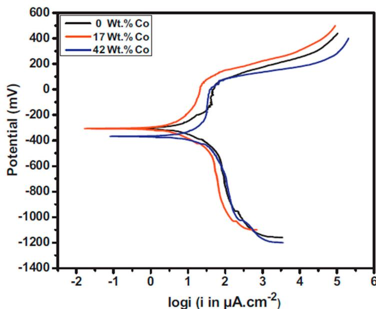
**Figure 13.** The potentiodynamic polarization curves of the Ni–Co alloy coating as a function of the cobalt content [126]. Reprinted from Applied Surface Science, 307, Babak Bakhit, Alireza Akbari, Farzad Nasirpour, Mir Ghasem Hosseini, Corrosion resistance of Ni–Co alloy and Ni–Co/SiC nanocomposite coatings electrodeposited by sediment codeposition technique/Pages No. 351–359, Copyright (2020), with permission from Elsevier.
