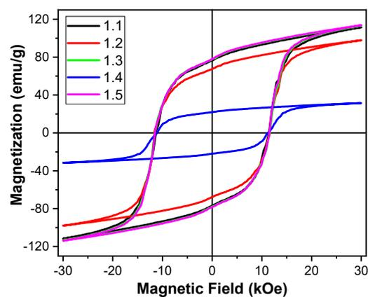
**Figure 8.** Magnetic hysteresis loop of AM fabricated NdFeB PPS bonded PM at room temperature. Sample ID: 1.1- as printed; 1.2-uncoated (dipped in pH 1.35 solution for 24 h), 1.3- coated with 3M ScotchWeld DP100 (dipped in pH 1.35 solution 24 h), 1.4- uncoated (80 °C; 95% RH; > 120 h), 1.5- coated with 3M ScotchWeld DP100 (80 °C; 95% RH; > 100 h).
