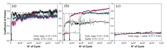
**Figure 2.** Evolution of coefficient of friction (COF) during test: (**a**) bulk sample, (**b**) 30% porosity, and (**c**) 60% porosity samples. Each curve is an independent measurement. The arrows indicate the duration of the early stage.
