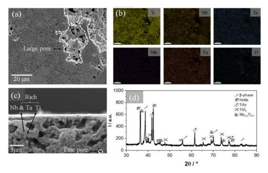
**Figure 1.** Microstructure and composition of as-sintered 30% porosity sample: (**a**) Top view FE-SEM micrograph, (**b**) Elemental mapping of the alloying elements in image (**a**), (**c**) Cross-section FE-SEM micrograph, and (**d**) XRD pattern with peaks marked with the corresponding phases.
