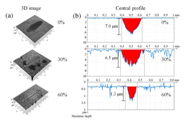
**Figure 3.** Images of wear tracks on the surface obtained by (**a**) optical profilometer for samples with different porosity and (**b**) the scratch profile after being tested.
