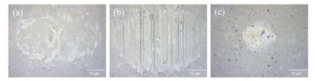
**Figure 4.** Optical images of the contact areas observed on the alumina balls after completing 100,000 test cycles on (**a**) bulk, (**b**) 30%, and (**c**) 60% porosity samples.
