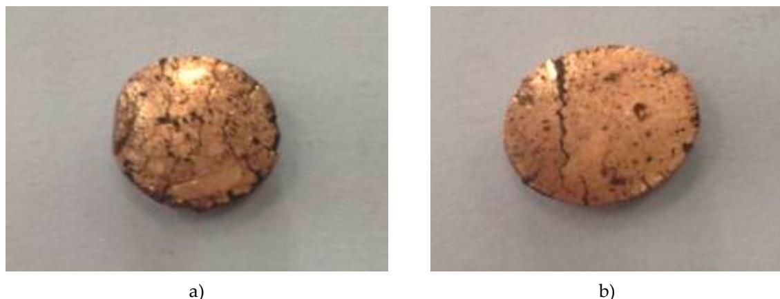
**Figure 19.** Images of Cu-5% $\text{Fe}_3\text{O}_4$  (a) and Cu-15% $\text{Fe}_3\text{O}_4$  (b) nanocomposites after cold rolling.
