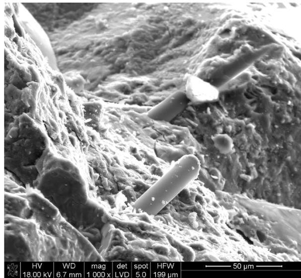
**Figure 19.** RPC microstructure. Visible parallel arrangement of basalt fibers.
