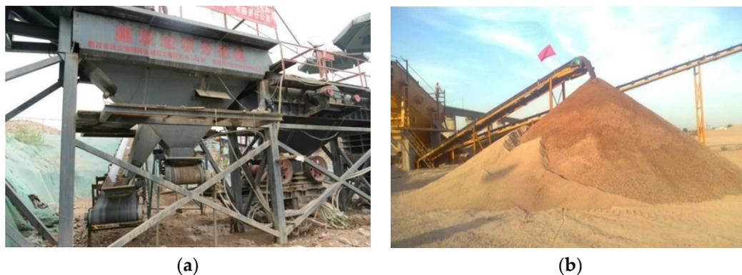
**Figure 16.** Brick separation technology and upgraded recycled aggregates production: (a) Brick separation device; (b) Purified recycled aggregate.
