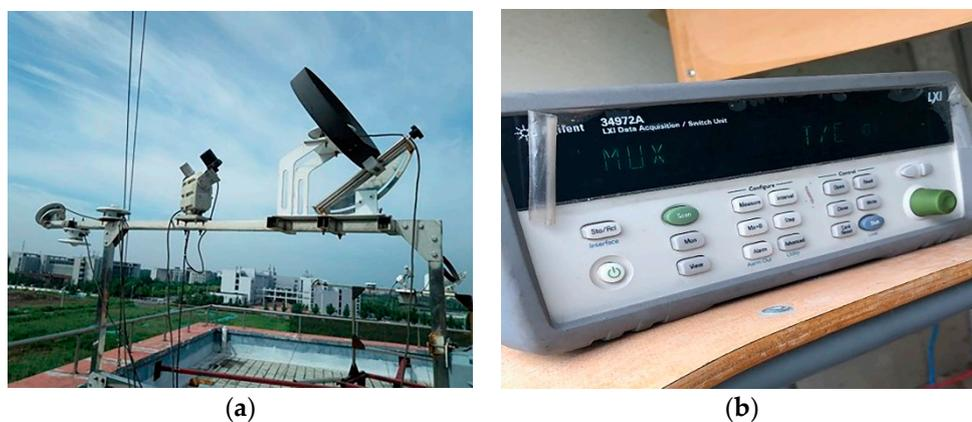
Figure 5. Main test equipment: (a) Weather station; (b) Data acquisition instrument.
