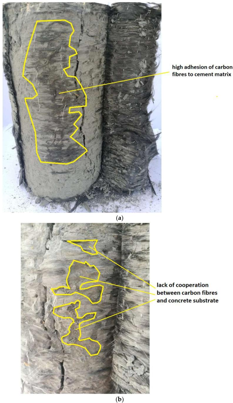
**Figure 11.** Analysis of the failure of the connection between the carbon fiber reinforced with the cement matrix and the sanded concrete surface: view of the entire sample (a) and enlargement of the extrusion area of the cement matrix (b).
