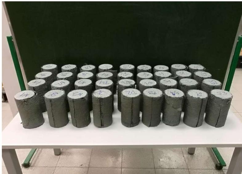
**Figure 9.** Concrete samples reinforced with carbon fibers using a cement matrix—state after the failure tests.
