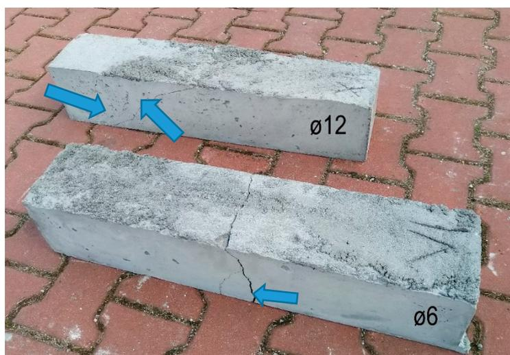
**Figure 10.** Small RC beams without transverse reinforcement—three-point bending test, with a span of 600 mm.
