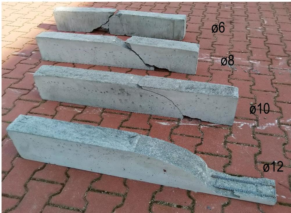
**Figure 12.** Reinforced concrete beams without transverse reinforcement after testing.
