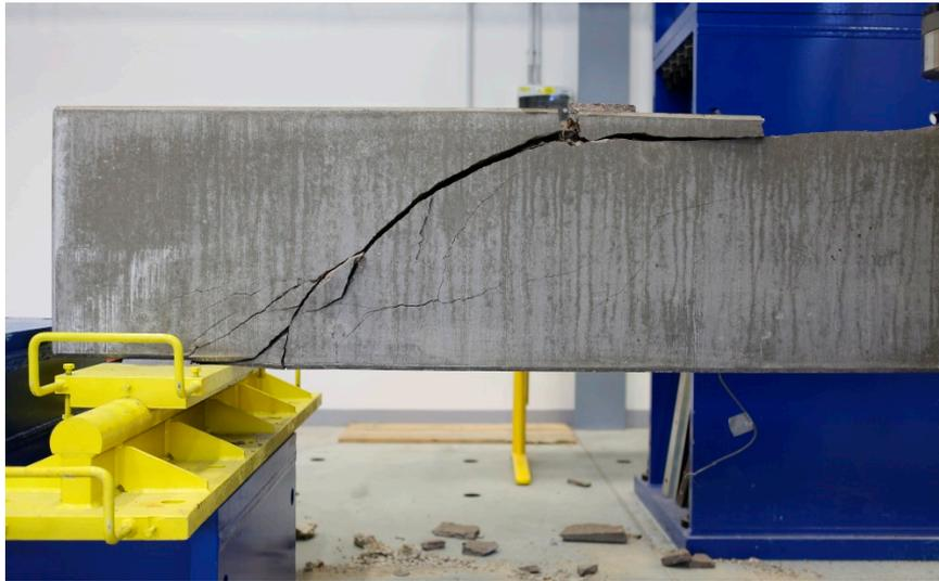
**Figure 7.** RC beams with transverse reinforcement (A1)—experimental program for material high-performance concrete (HPC).
