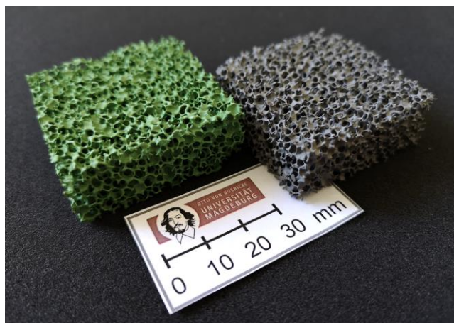
Figure 1. Specimens of NiO–YSZ (left) and Ni–YSZ cellular composites (right). The ratio of NiO and YSZ is 1:1 by weight. Before reduction, the foams possess the typical green color of NiO, which transforms to grey after reduction to metallic Ni.
